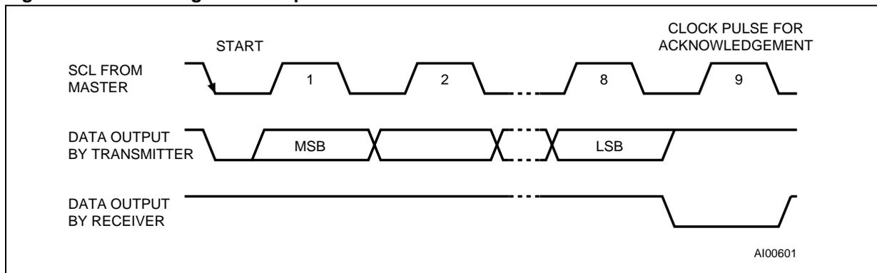
Figure 10. Bus Timing Requirements Sequence
