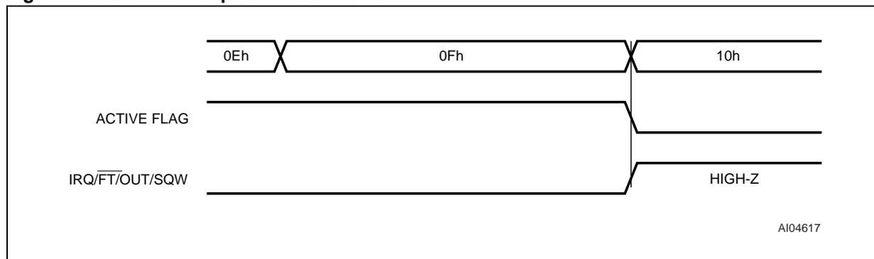
**Figure 17. Back-up Mode Alarm Waveform**
