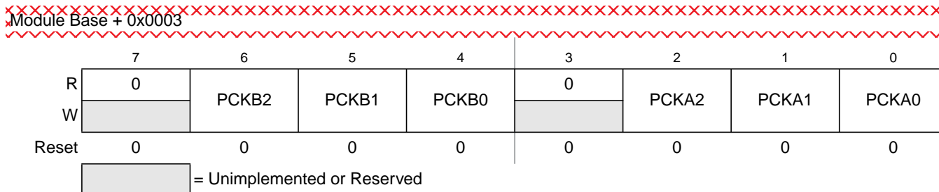
Figure 10-6. PWM Prescaler Clock Select Register (PWMPRCLK)
