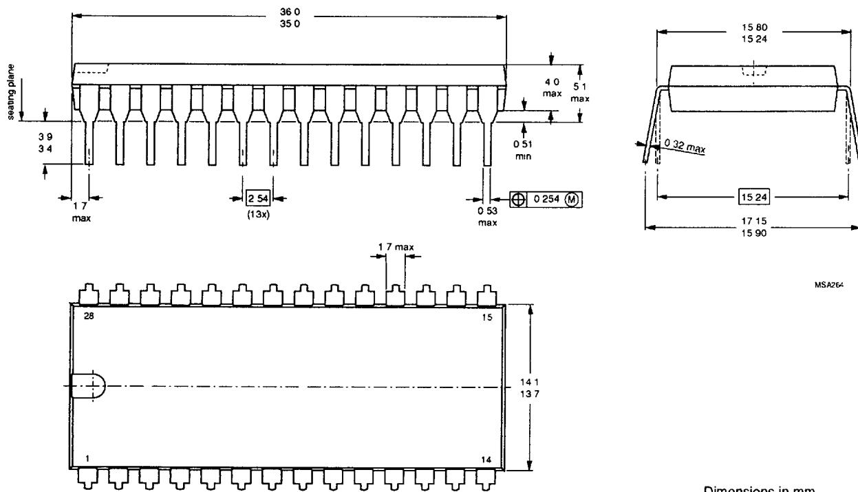
Fig.5 28-lead dual in-line; plastic (SOT117).
