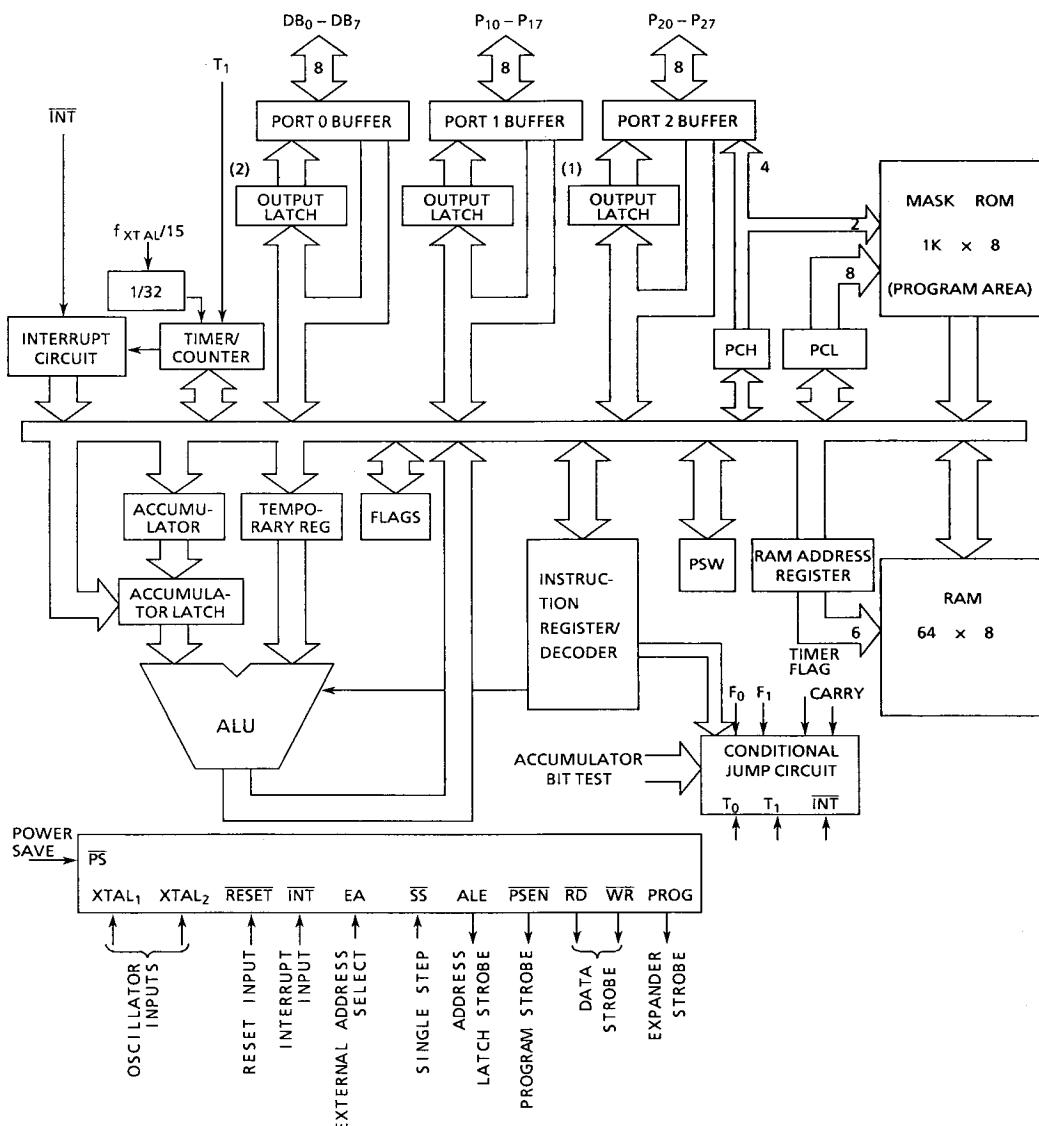
Note 1 : The lower order 4 bit of port 2 output latch are used also for input/output operations with the I/O expander.
