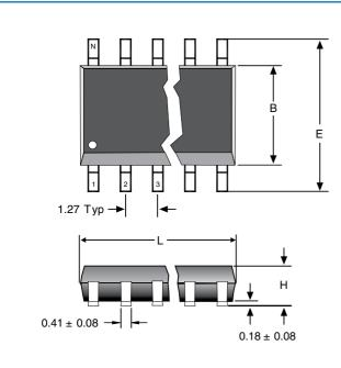
Note: All dimesions exclude mold flash and end flash which shall not exceed 0.15 per side.
