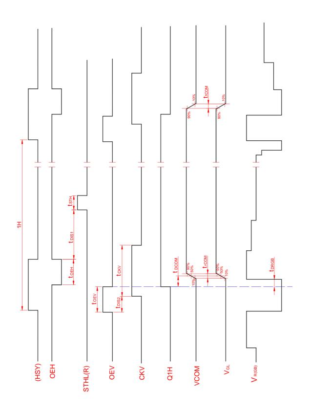
Fig.4-(b) Detail horizontal timing
