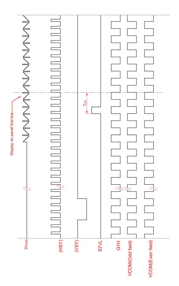
Fig.6-(a) Vertical timing (From up to down)
