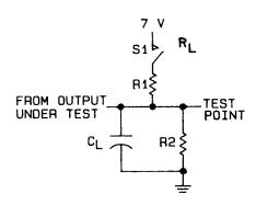
NOTE:  $C_L = 50$  pF, includes probe and jig capacitance.  $R_L = R1 = R2 = 500 \Omega_{\odot}$
