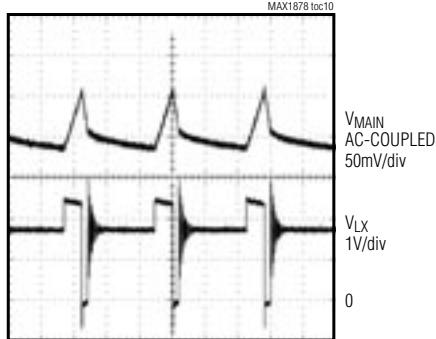
STEP-DOWN LIGHT-LOAD SWITCHING WAVEFORMS
