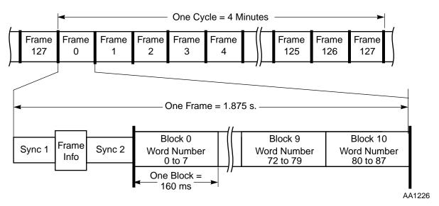
Figure A-1 FLEX™ Signal Structure
