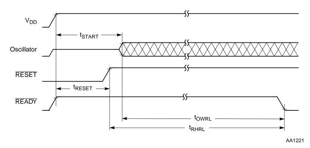
Figure 2-1 Startup Timing
