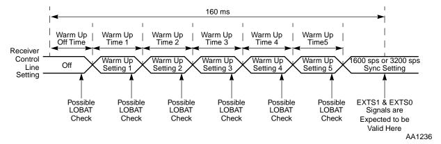
Figure C-1 Automatic Receiver Warm Up Sequence
