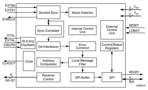
Figure 1 MC68181 Functional Block Diagram
