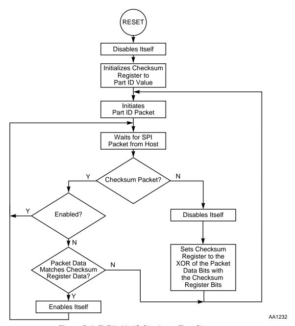
Figure B-4 FLEX chip IC Checksum Flow Chart
