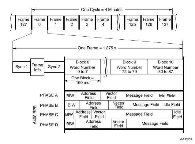
Figure A-4 FLEX™ Signal Structure For 6400 BPS
