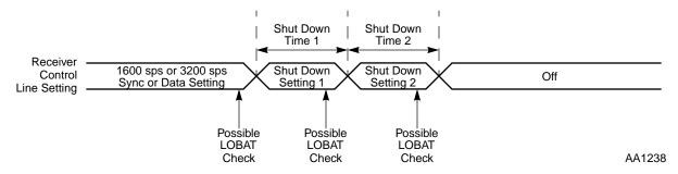
Figure C-3 Receiver Shut Down Sequence
