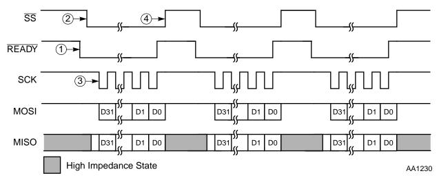
Figure B-1 Typical Multiple Packet Communications Initiated by the Host
