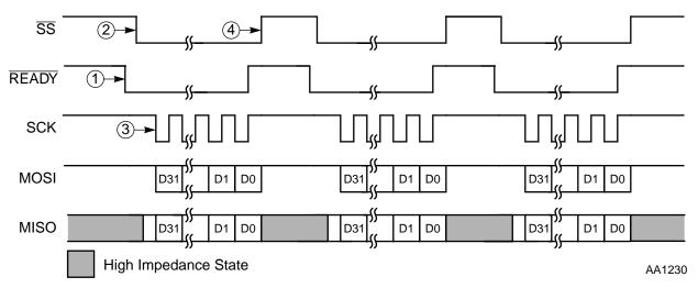
Figure B-2 Typical Multiple Packet Communications Initiated by the FLEX chip IC
