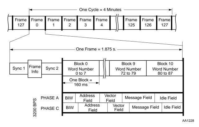
Figure A-3 FLEX™ Signal Structure for 3200 BPS
