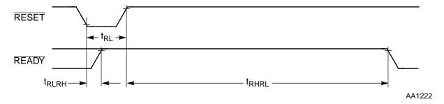
Figure 2-2 Reset Timing
