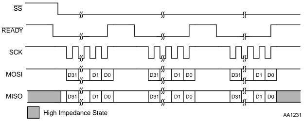
Figure B-3 Multiple Packet Communications Initiated by the FLEX chip IC with No De-select
