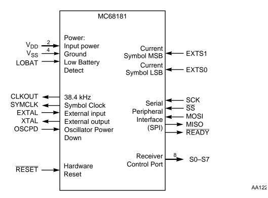
Figure 1-1 Signals Identified by Functional Group
