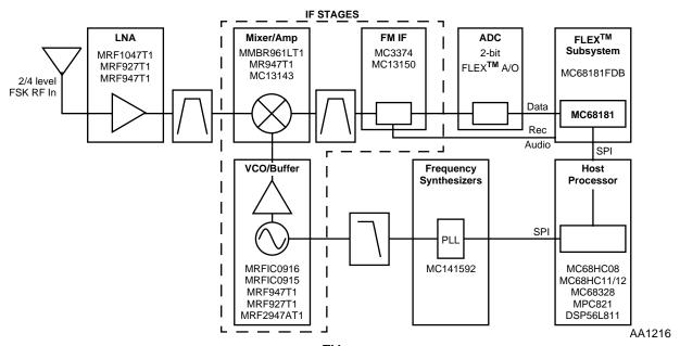
Figure 4-1 Roaming FLEX<sup>TM</sup> chip System Block Diagram
