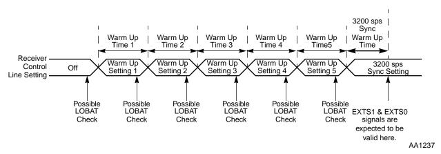
Figure C-2 Host Initiated Receiver Warm Up Sequence
