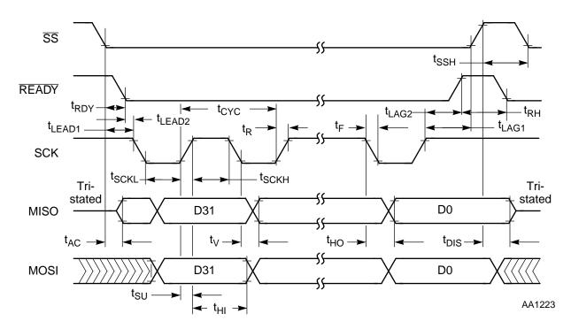
Figure 2-3 SPI Timing
