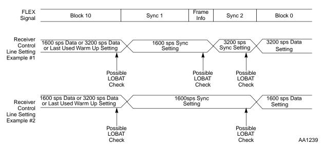
Figure C-4 Examples of Receiver Control Transitions
