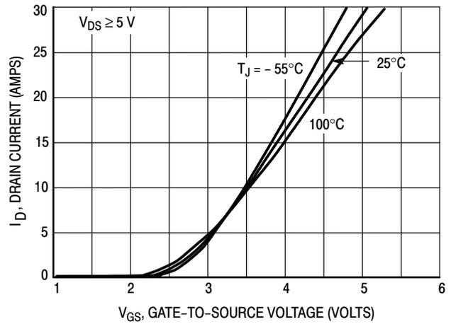
Figure 2. Transfer Characteristics
