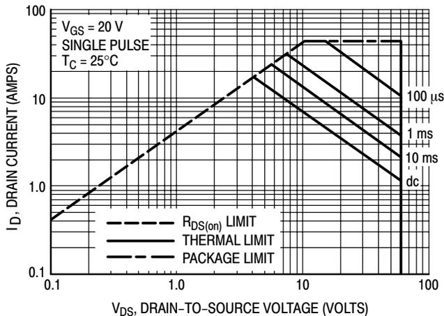
Figure 12. Maximum Rated Forward Biased Safe Operating Area
