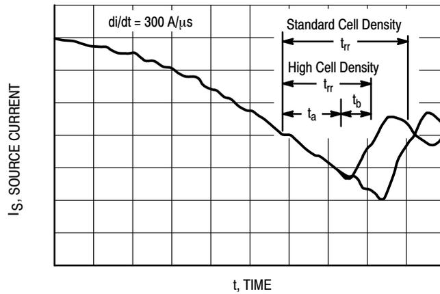
Figure 11. Reverse Recovery Time ( $t_{rr}$ )
