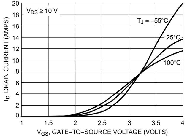
Figure 2. Transfer Characteristics
