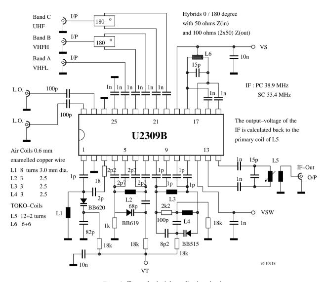
Figure 2. Test and principle application circuit
