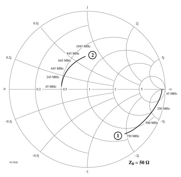
Figure 4. Input impedance mixer band A (S11A), B and C (S11B/C)
