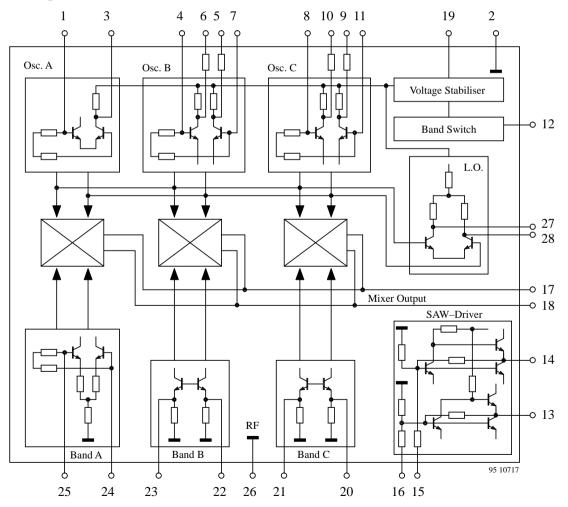
Figure 1. Block diagram pinning of U2309B
