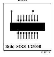
Figure 3. PCB for the  $R_{thJA}$ -measurement
