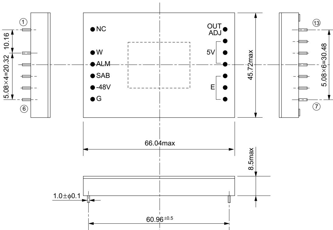
\* Dimensions are in millimeters.
