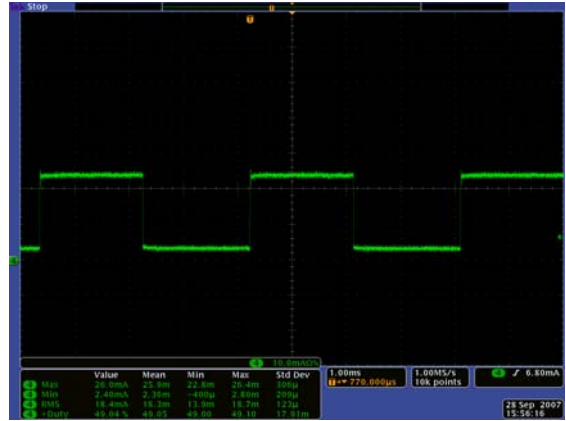
FIGURE 15. I LED AT 50% PWM DIMMING
