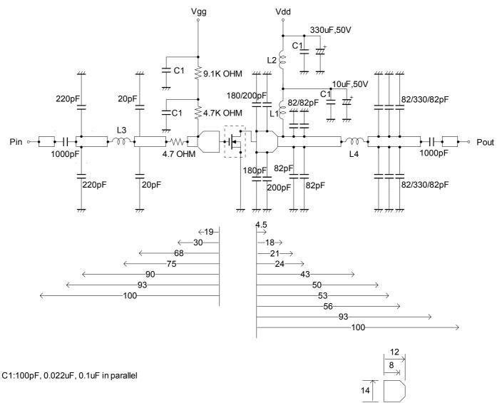
L1:8Turns,I.D8mm,D1.6mm silver plateted copper wire L2:10Turns,I.D8mm,D1.6mm silver plateted copper wire L3:5Turns,I.D6mm,D0.7mm copper wire P=1mm L4:1Turns,I.D10mm,D1.6mm silver plateted copper wire Dimensions:mm
