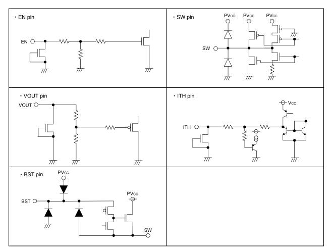
Fig.34 I/O equivalence circuit
