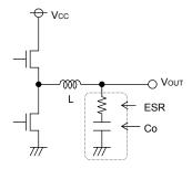
Fig.28 Output capacitor
