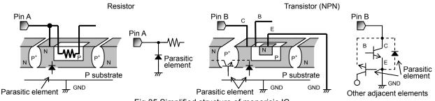
Fig.35 Simplified structure of monorisic IC
