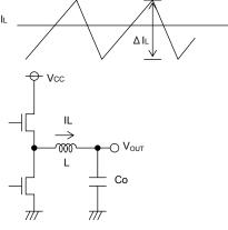
Fig.27 Output ripple current
