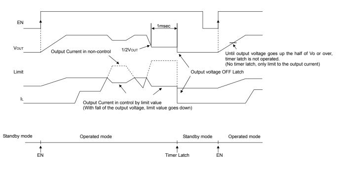
Fig.25 Short-current protection circuit with time delay timing chart
