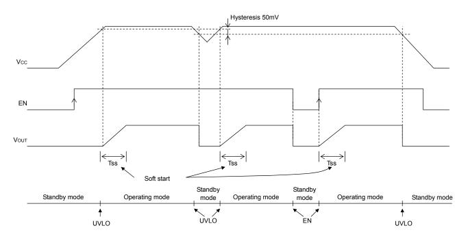
Fig.24 Soft start, Shutdown, UVLO timing chart
