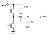
Fig.29 Input capacitor
