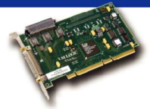
The LSIU160 Ultra160 SCSI host adapter is the best solution to connect to high performance Ultra160 hard disks drives.
