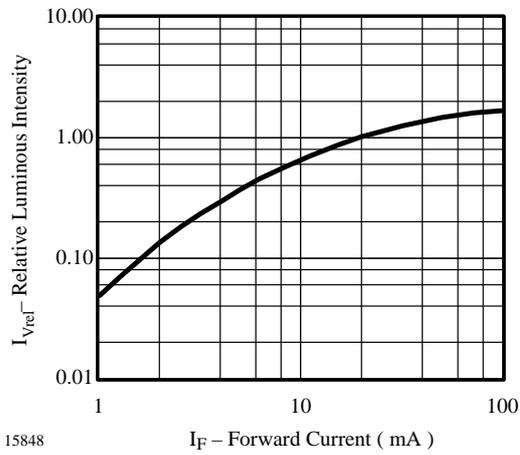
Figure 6. Relative Luminous Intensity vs. Forward Current
