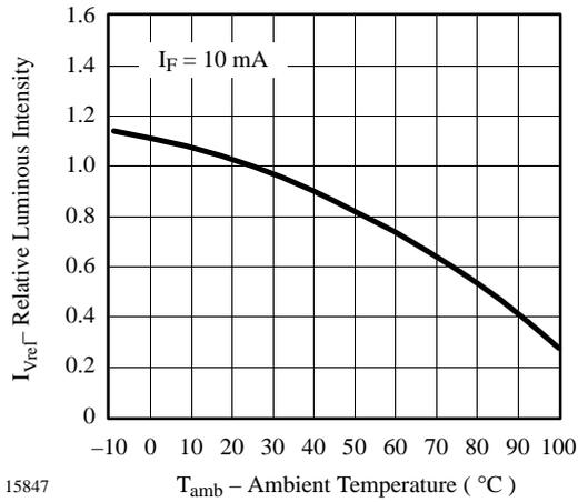
Figure 5. Rel. Luminous Intensity vs. Ambient Temperature
