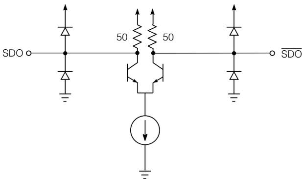
Fig. 5 Serial Data Outputs
