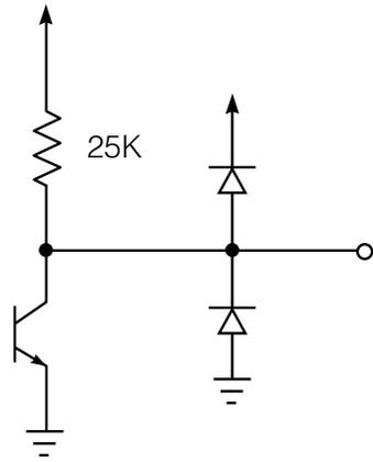
Fig. 7 Indicator Outputs: HD/ $\overline{SD}$ , LD
