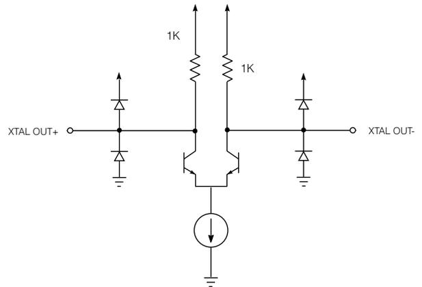
Fig. 4 Crystal Output Buffer
