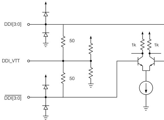
Fig. 9 Serial Data Inputs
