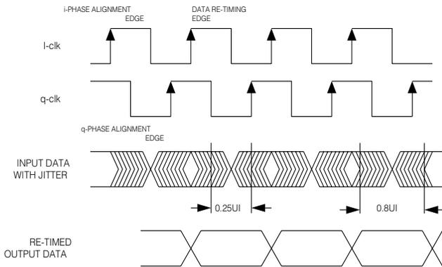
Fig. 11 Phase Detector Characteristics.
