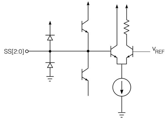
Fig. 8 Standard Select/Indication Bi-directional pins
