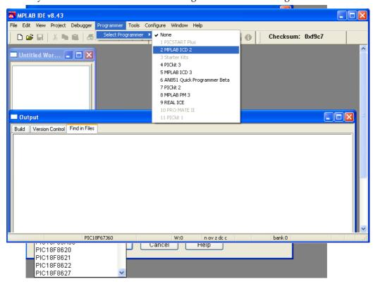
Wait while MPLAB is downloading operation system, and after ICD2 is connected – check in menu Programmer – Settings – Power – there is option – Power target circuit from MPLAB ICD 2 –
