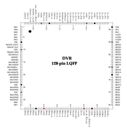
Figure 3.1 W9980D Pin configuration
