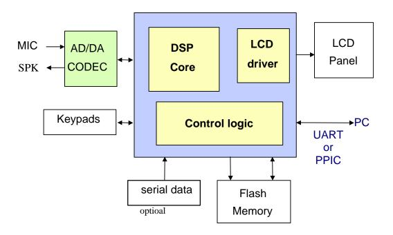
Figure 5.1 W9980D-Based Digital Voice Recorder System Diagram
