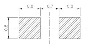
**Note:** Tolerances Unless Dimension is  $\pm 0.1$ mm, Unit = mm
