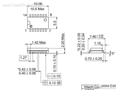
\*Dimension including the plating thickness
