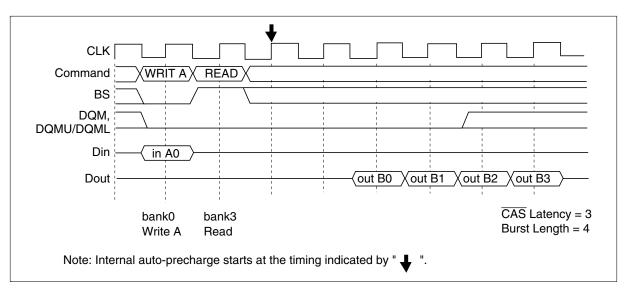
**2.** Same bank: The consecutive read command from write with auto precharge (the same bank) is illegal. It is necessary to separate the two commands with a bank active command.
