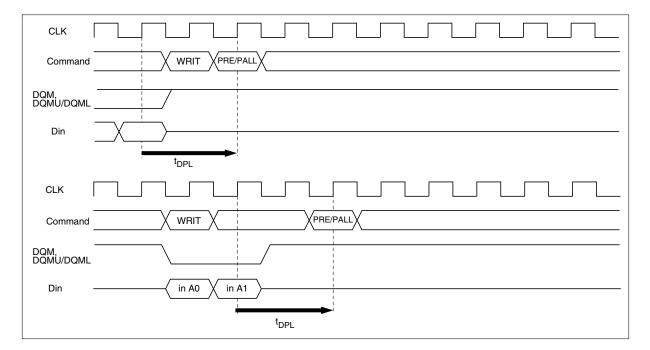
**Burst Length = 4** (To stop write operation)
