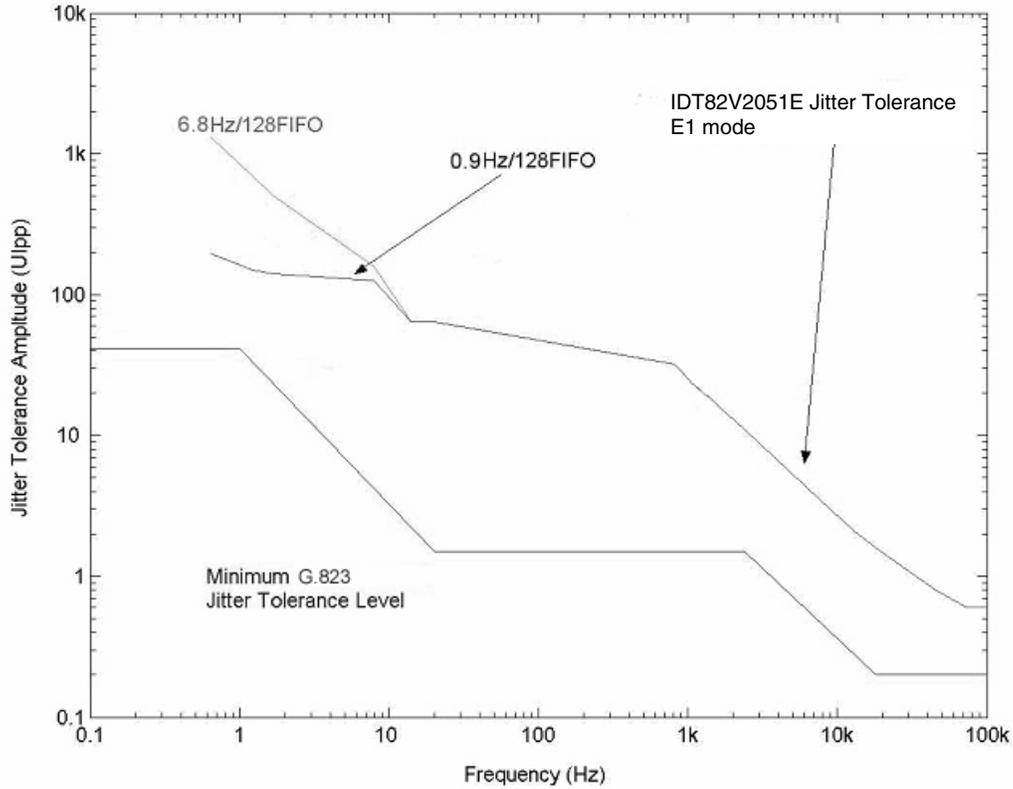
Figure-19 E1 Jitter Tolerance Performance
