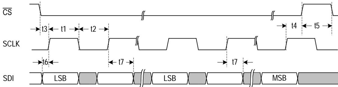
Figure-21 Serial Interface Write Timing
