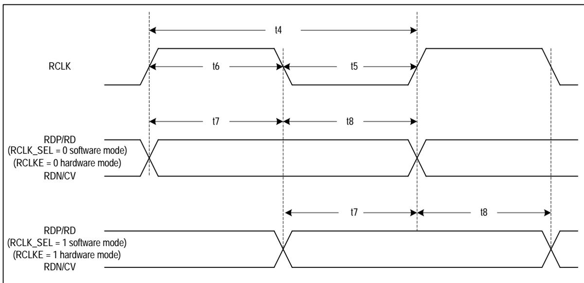
**Figure-18 Receive System Interface Timing**
