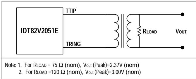
Figure-3 E1 Pulse Template Test Circuit
