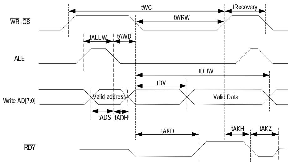
Figure-27 Multiplexed Intel Write Timing
