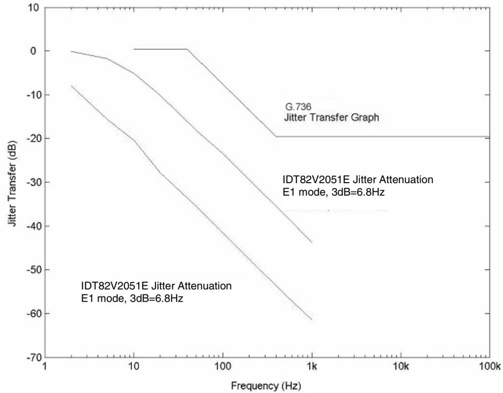
**Figure-20 E1 Jitter Transfer Performance**
