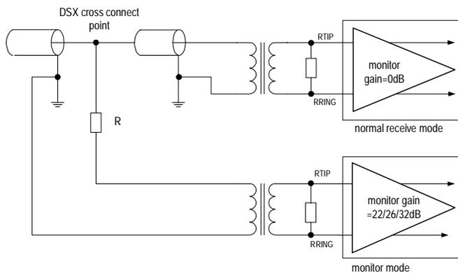
**Figure-6** Monitoring Receive Line in Another Chip
