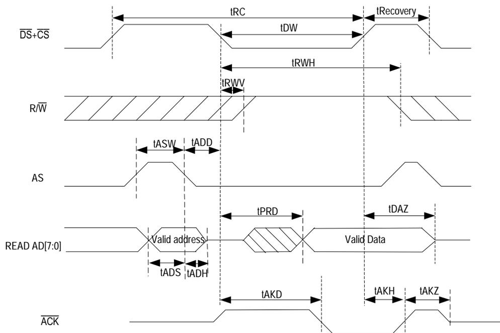
Figure-24 Multiplexed Motorola Read Timing
