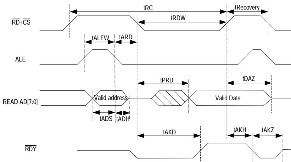
Figure-26 Multiplexed Intel Read Timing
