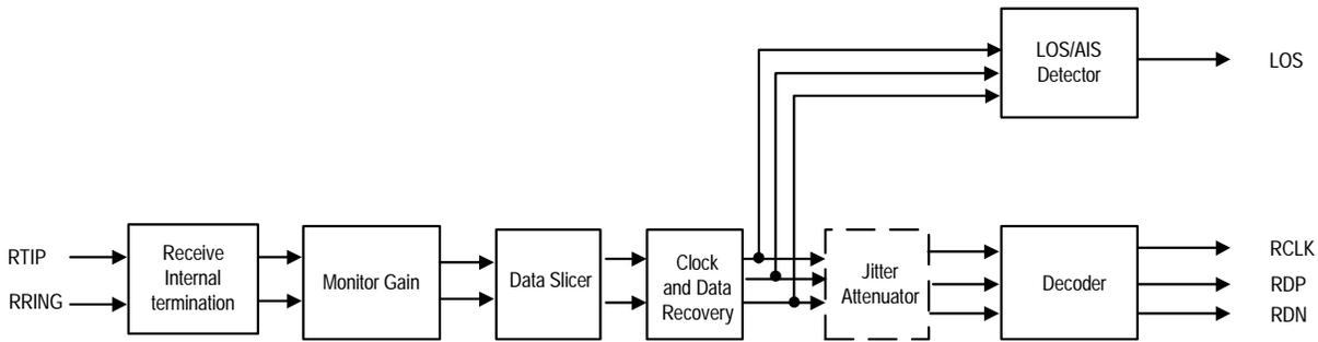
Figure-4 Receive Path Function Block Diagram
