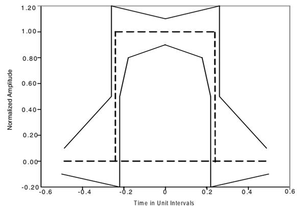
Figure-2 E1 Waveform Template Diagram
