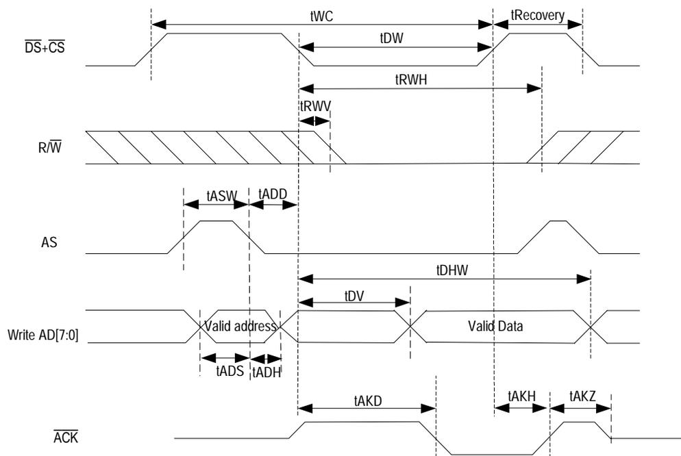
Figure-25 Multiplexed Motorola Write Timing
