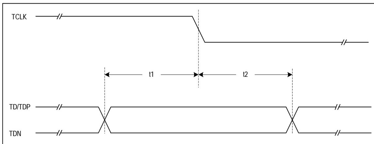
Figure-17 Transmit System Interface Timing
