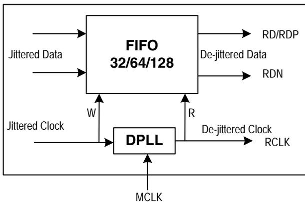
**Figure-8 Jitter Attenuator**
