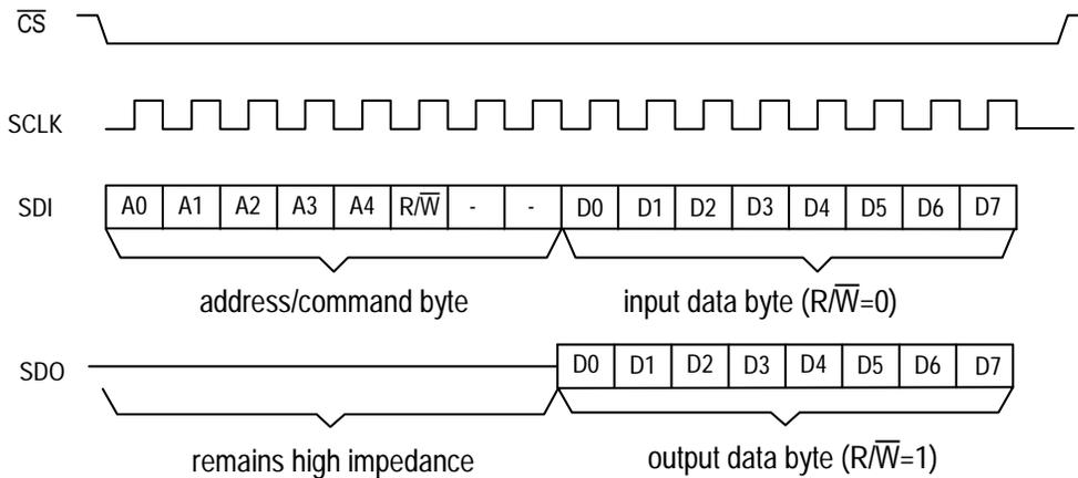
**Figure-16 Serial Microcontroller Interface Function Timing**
