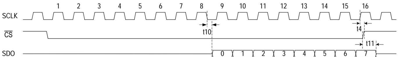
Figure-22 Serial Interface Read Timing with SCLKE=1
