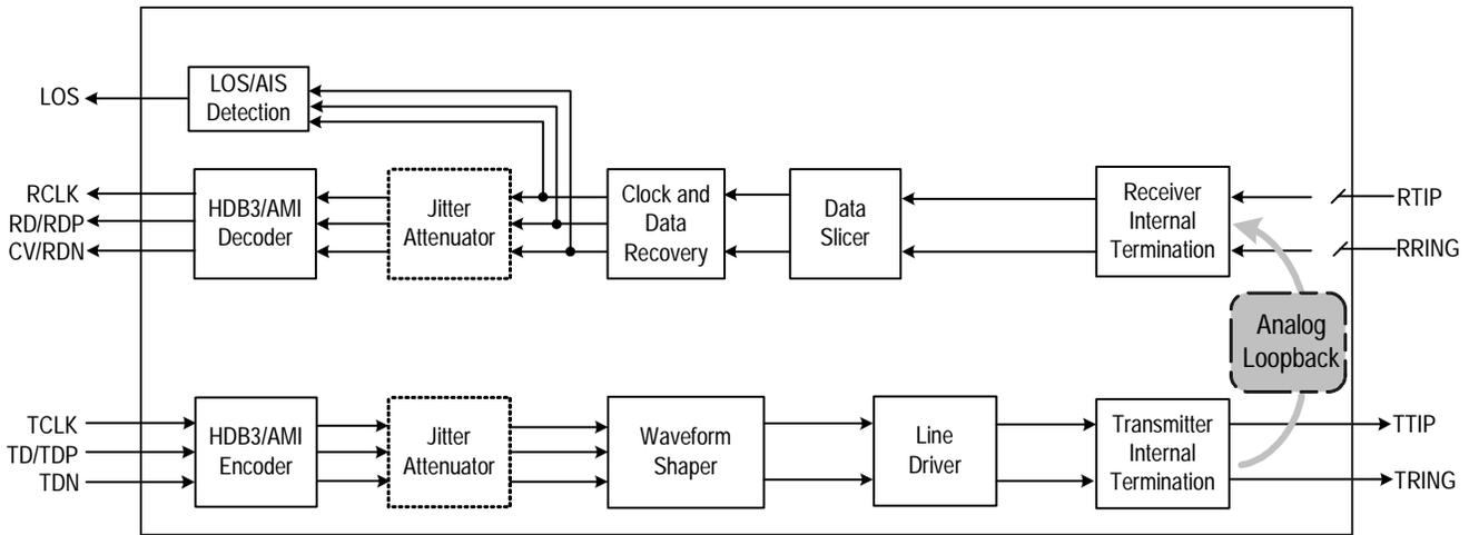
Figure-10 Analog Loopback
