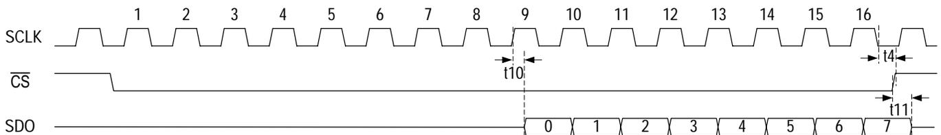
Figure-23 Serial Interface Read Timing with SCLKE=0
