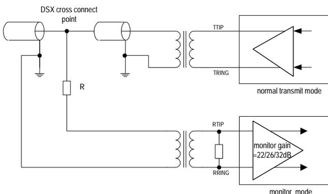
**Figure-7** Monitor Transmit Line in Another Chip
