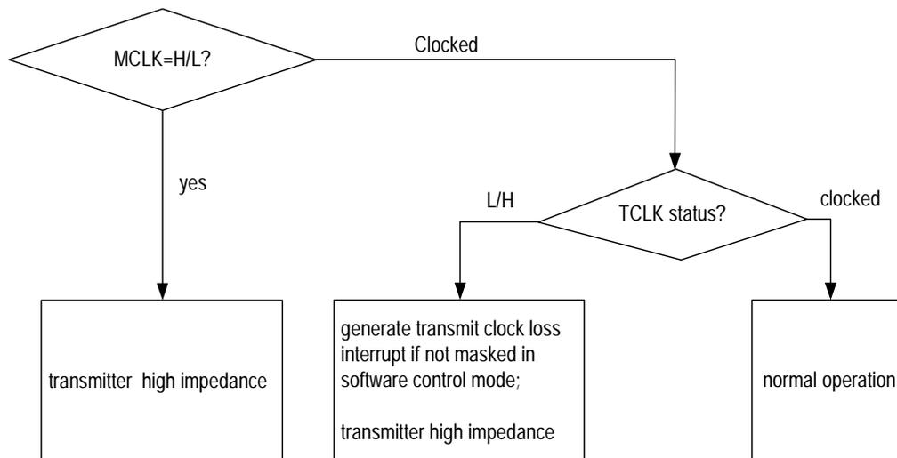
**Figure-15 TCLK Operation Flowchart**
