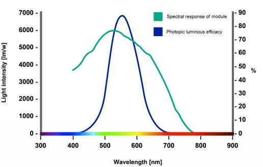
G24i's dye sensitised indoor photovoltaic modules have been optimised to work under indoor lighting providing the highest power density.
