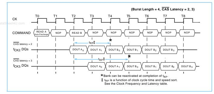
If interrupting a Read Command with auto-precharge with a Write Command, DQM must be used to avoid DQ contention.
