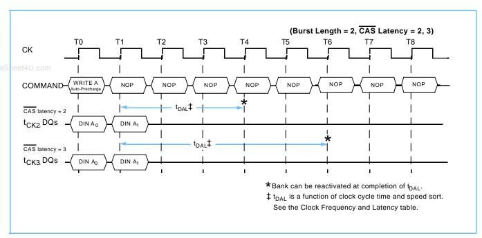
Similar to the Read Command, a Write Command with auto-precharge can not be interrupted by a command to the same bank. It can be interrupted by a Read or Write Command to a different bank, however. The interrupting command will terminate the write. The bank undergoing auto-precharge can not be reactivated until t<sub>DAI</sub> is satisfied.
