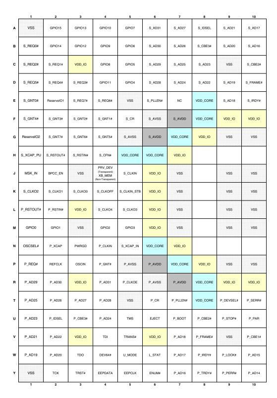
Figure 26-2. PCI 6540 Physical Layout with Pinout—Topside View (A1-A10 through Y1-Y10)
