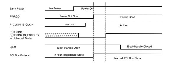
Figure 22-1. Hot Insertion Power-Up Sequence Recommendation
