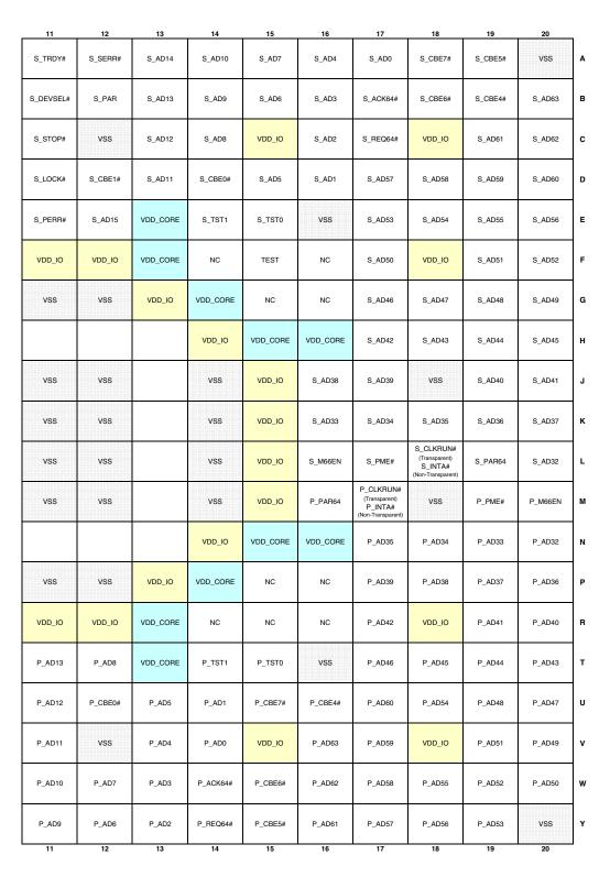
Figure 26-3. PCI 6540 Physical Layout with Pinout—Topside View (A11-A20 through Y11-Y20)
