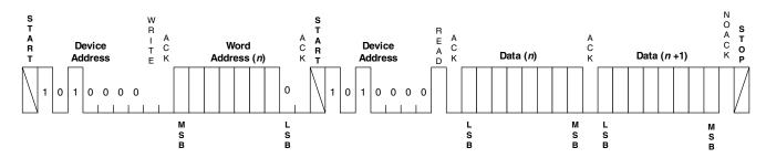
Figure 7-1. Serial EEPROM Data Structure
