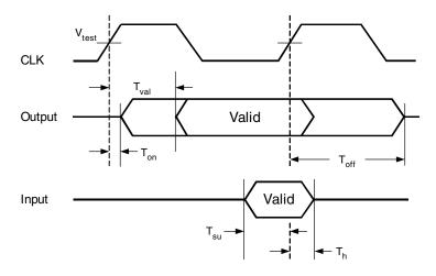
Figure 25-1. PCI-X/PCI Signal Timing Specification
