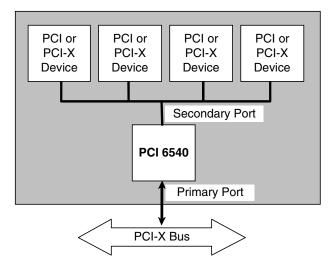
Figure 1-3. Multiple Device Expansion
