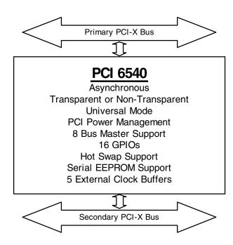
Figure 1-2. PCI 6540 PCI-X-to-PCI-X Bridge
