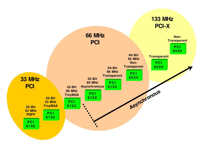
Figure 1-1. PCI 6000 Series of PCI-to-PCI Bridges
