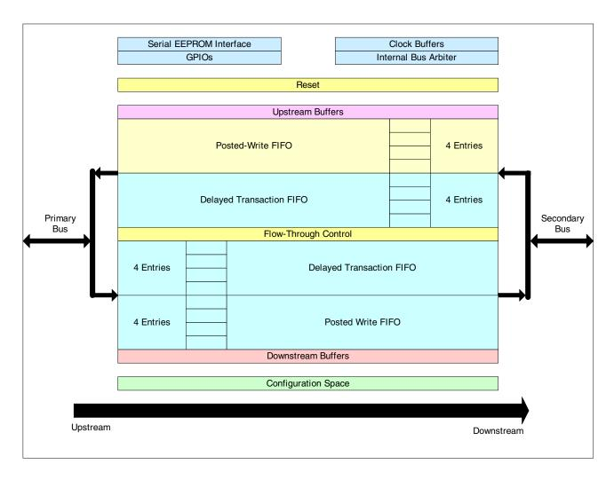
Figure A-1. PCI 6540 Internal Architecture
