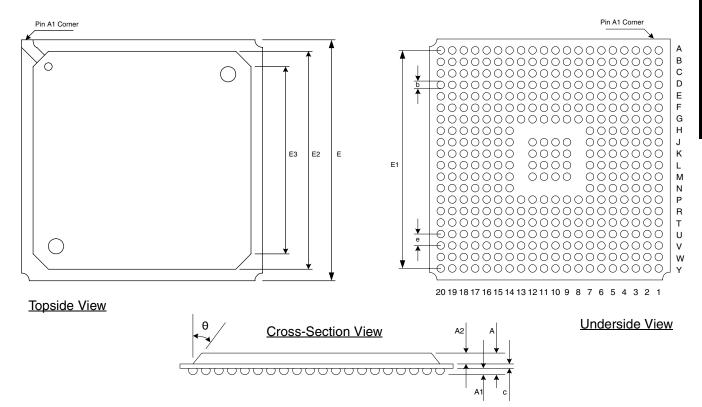
Figure 26-1. PCI 6540 Mechanical Dimensions
