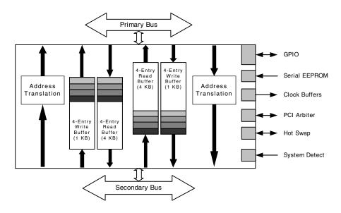
Figure 2-1. PCI 6540 Block Diagram
