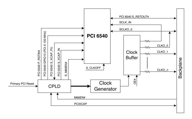
Figure B-1. CPLD Used to Detect Bus Type and Speed and Feed to PCI 6540 during Reset Phase
