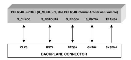
Figure A-5. Universal Mode Connections Example
