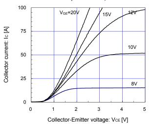
$[Inverter\ ] \\ Collector-Emitter\ voltage\ \ vs.\ Gate-Emitter\ voltage\ (typ.) \\ Tj=25^{\circ}C\ /\ chip$
