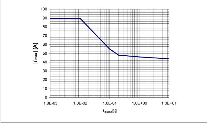
Figure 4 BTN7975B Maximum Single Pulse Current ( $T_c < 85^{\circ}C$ )
