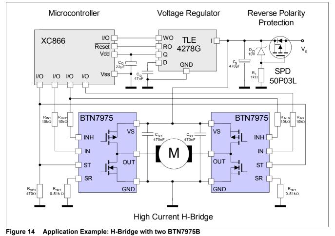
Note: This is a simplified example of an application circuit. The function must be verified in the real application.
