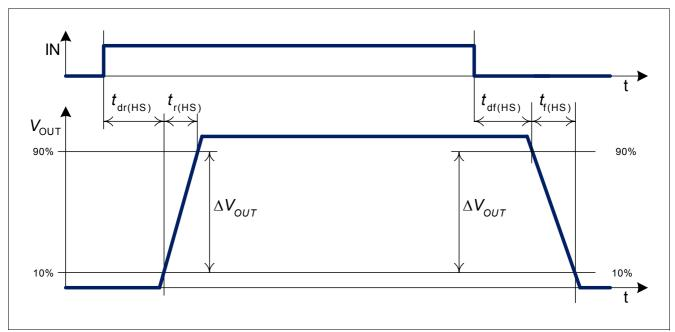
Figure 7 Definition of switching times high side (R<sub>load</sub> to GND)
