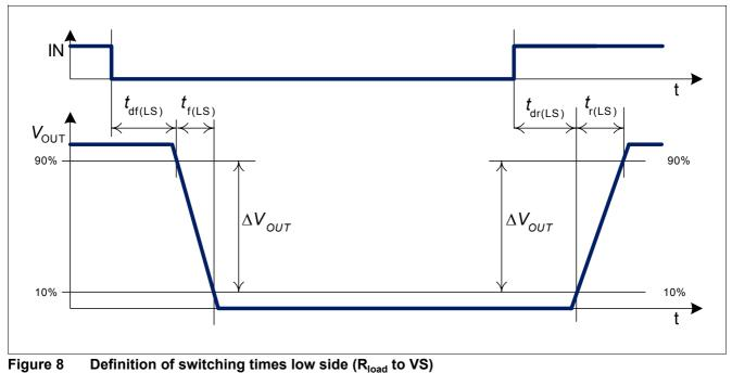
Due to the timing differences for the rising and the falling edge there will be a slight difference between the length of the input pulse and the length of the output pulse. It can be calculated using the following formulas:
