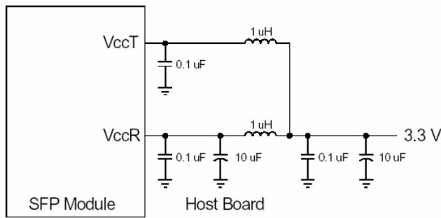
Figure 1, Recommended Host Board Power Supply Circuit
