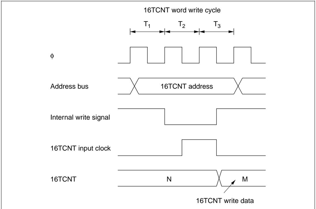
**Figure 9.38 Contention between 16TCNT Word Write and Increment**
