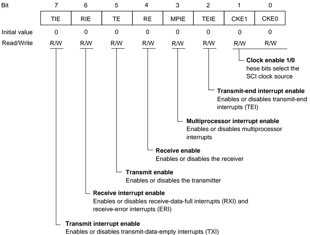
The CPU can always read and write SCR. SCR is initialized to H'00 by a reset and in standby mode.
