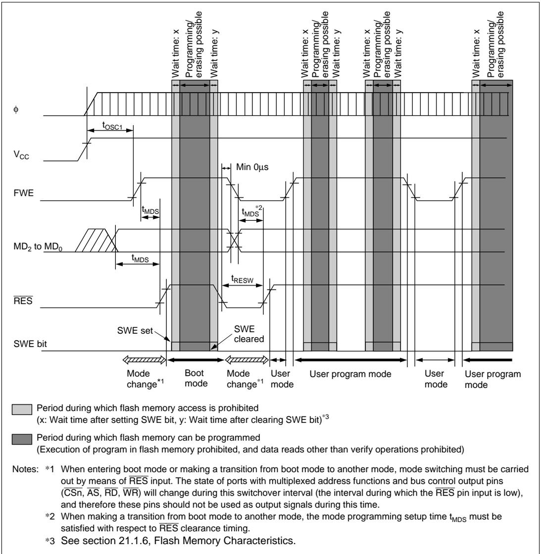
**Figure 18.18 Mode Transition Timing**
