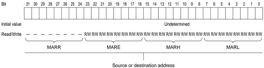
An MAR functions as a source or destination address register depending on how the DMAC is activated: as a destination address register if activation is by a receive-data-full interrupt from serial communication interface (SCI) channel 0 or by an A/D converter conversion-end interrupt, and as a source address register otherwise.
