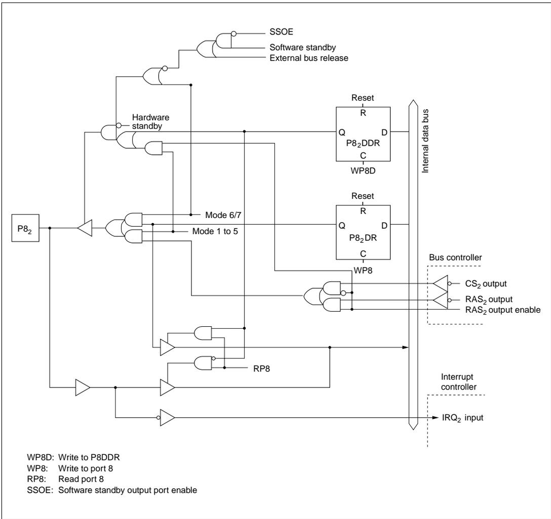
**Figure C.8 (c) Port 8 Block Diagram (Pin P8<sub>2</sub>)**
