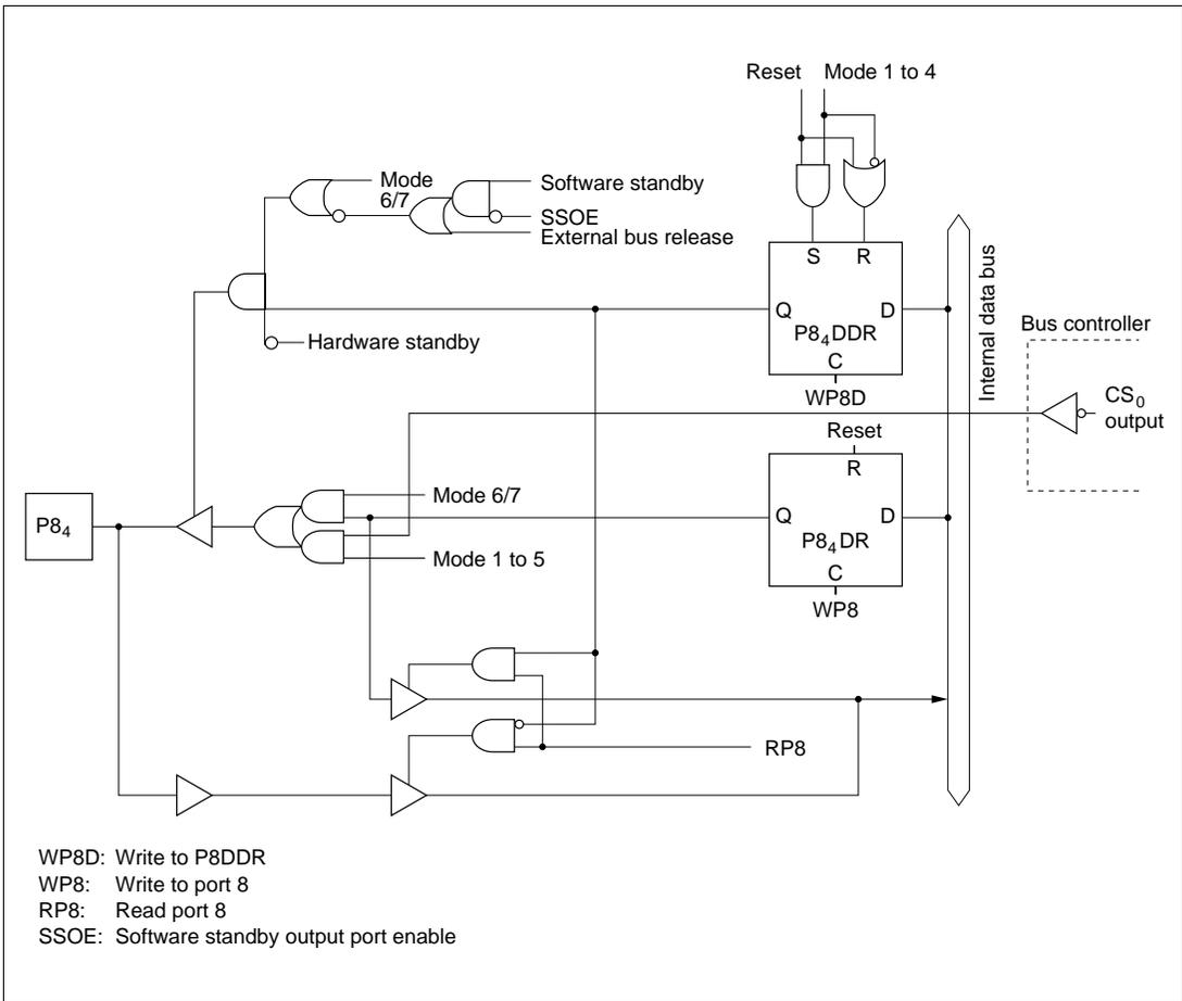
**Figure C.8 (e) Port 8 Block Diagram (Pin P84)**
