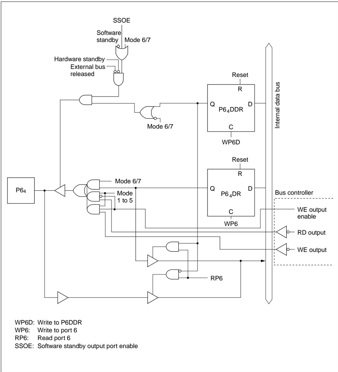
Figure C.6 (e) Port 6 Block Diagram (Pin P64)
