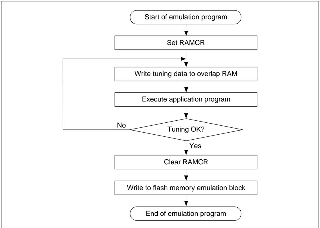
**Figure 18.13** Flowchart of Flash Memory Emulation in RAM
