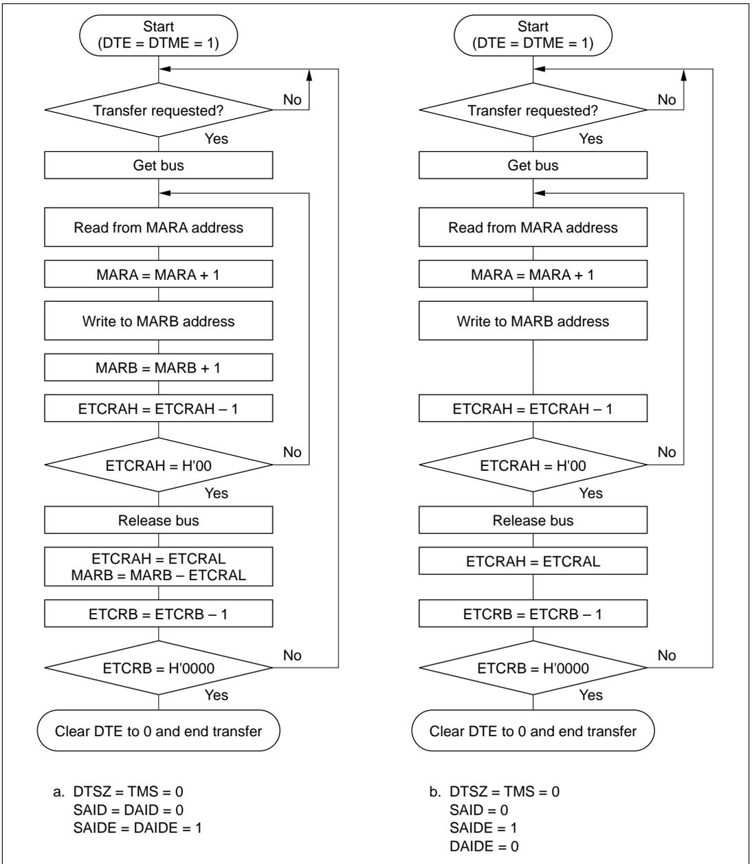
**Figure 7.11 Block Transfer Mode Flowcharts (Examples)**
