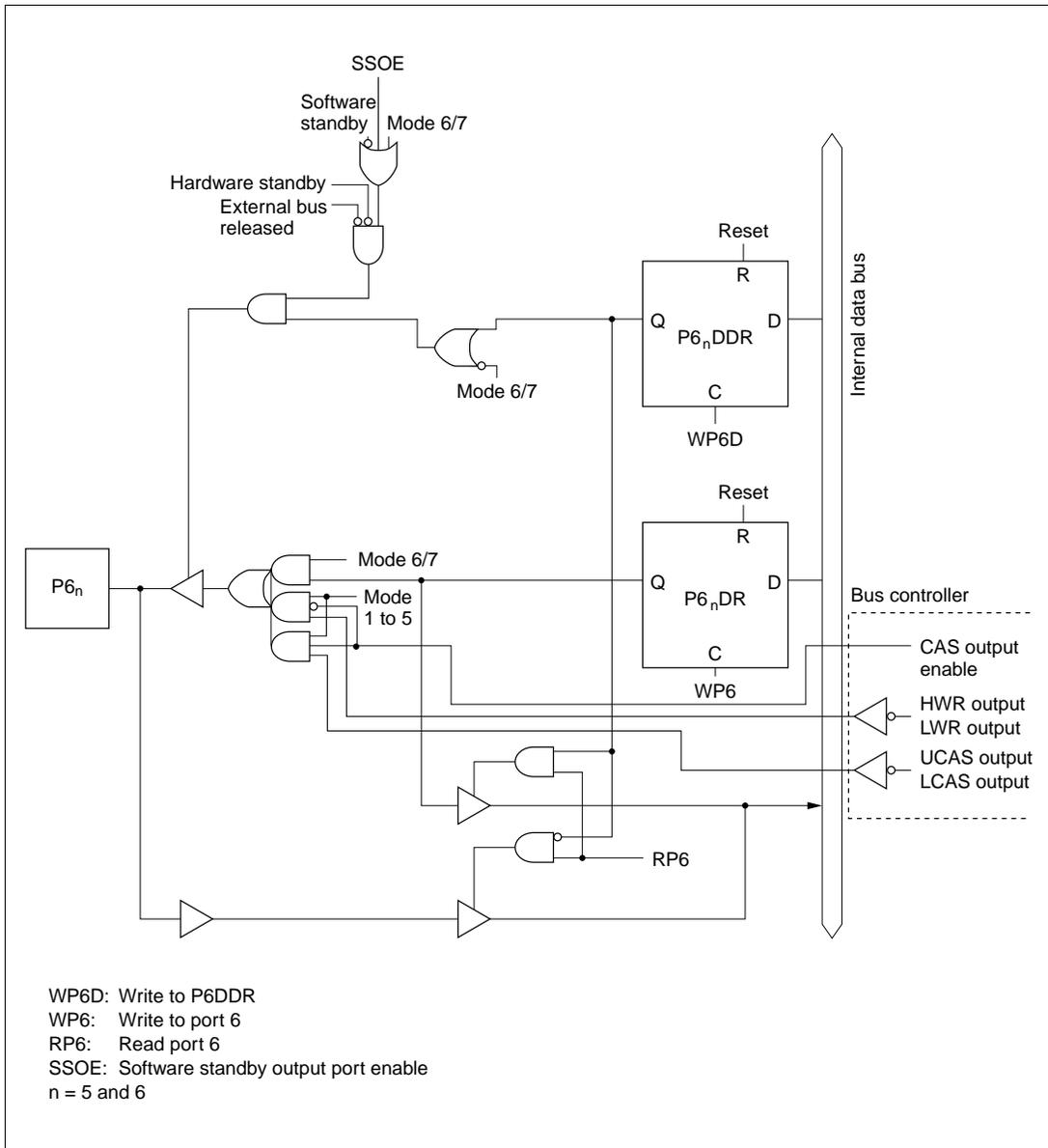
**Figure C.6 (f) Port 6 Block Diagram (Pins P6<sub>5</sub> and P6<sub>6</sub>)**
