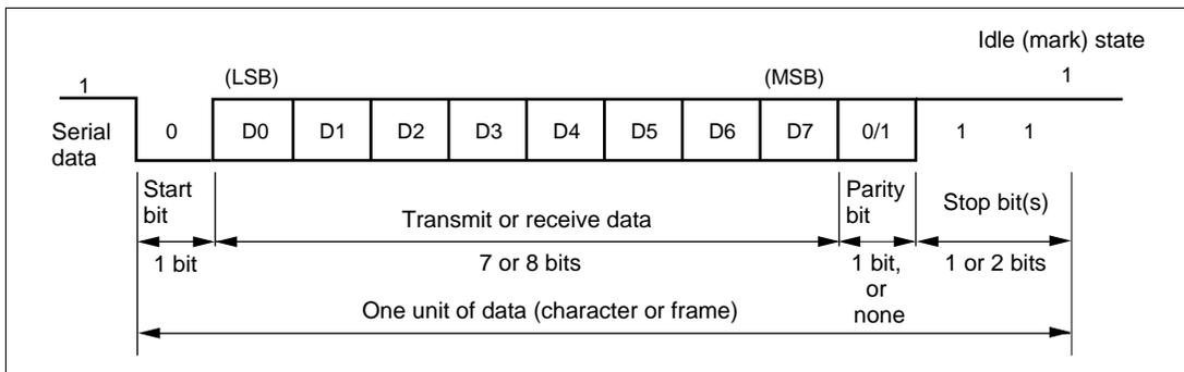
**Figure 13.2 Data Format in Asynchronous Communication
