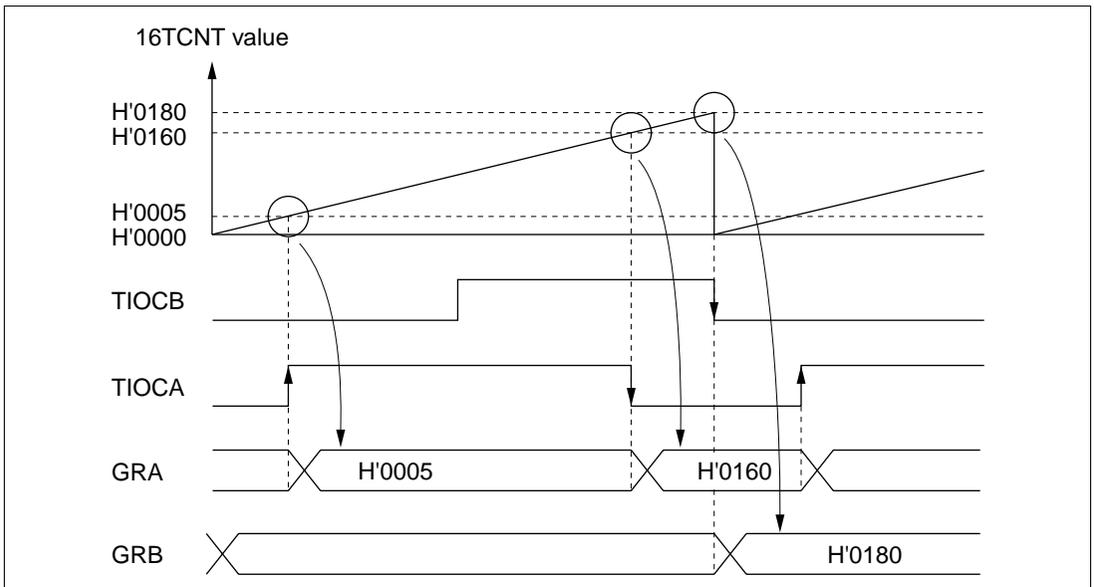
**Figure 9.22 Input Capture (Example)**
