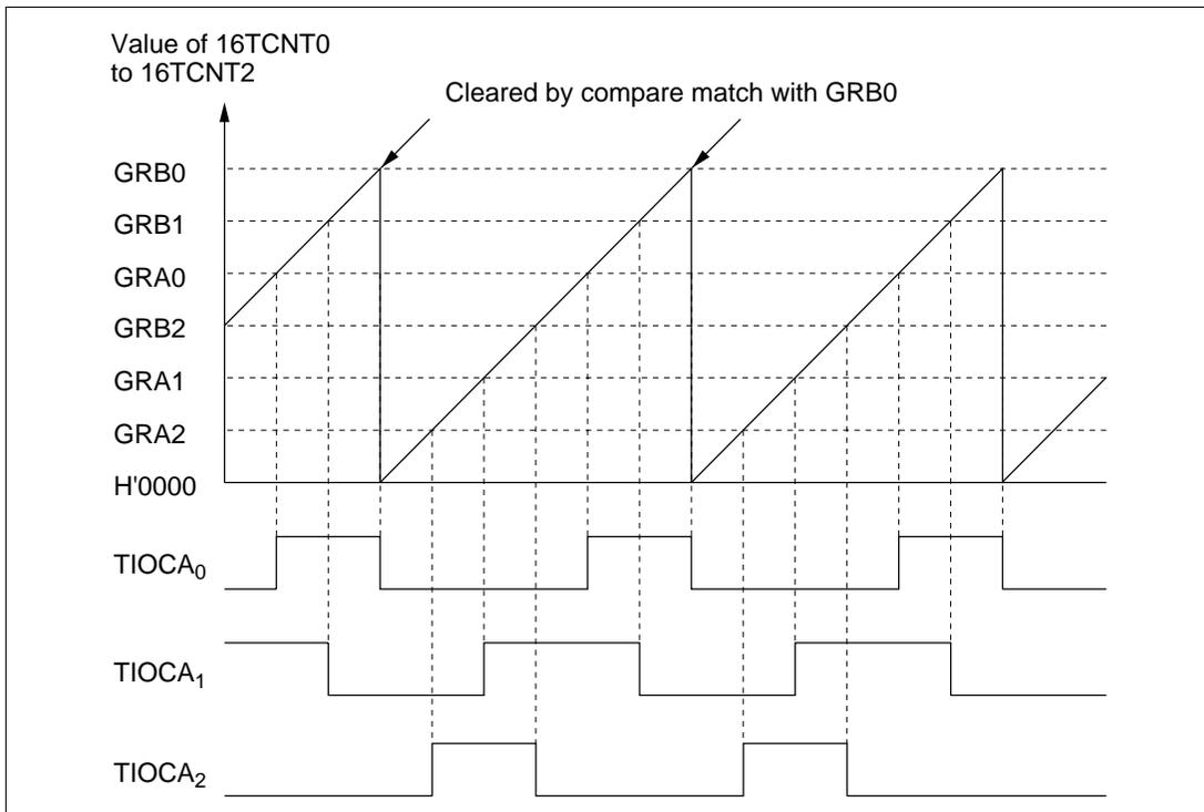
**Figure 9.25 Synchronization (Example)**
