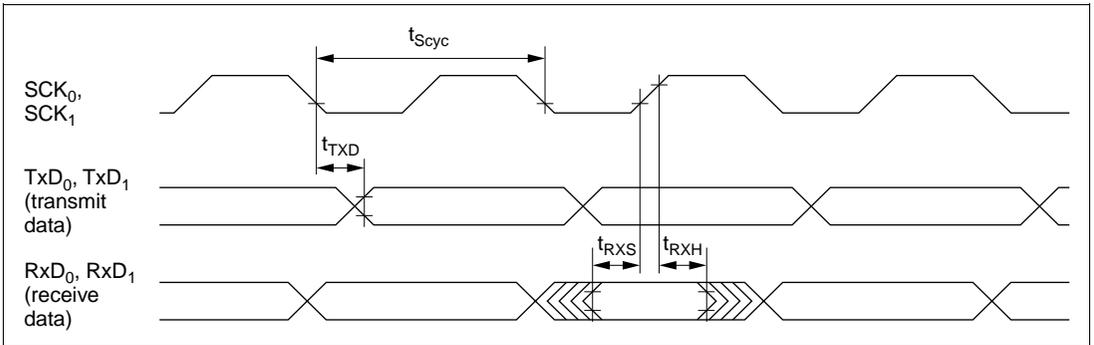
Figure 21.21 SCI Input/Output Timing in Synchronous Mode
