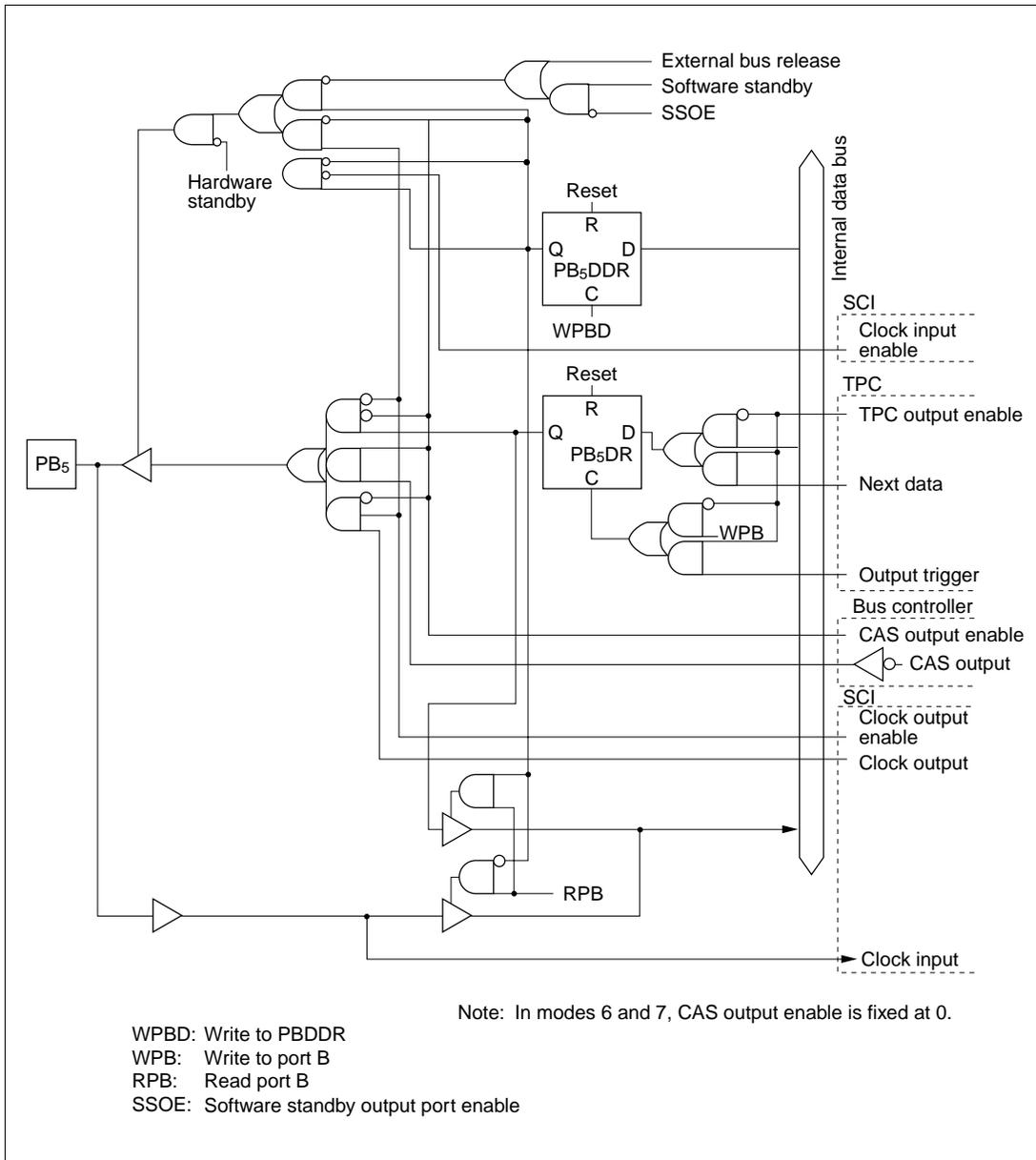
**Figure C.11 (f) Port B Block Diagram (Pin PB<sub>5</sub>)**
