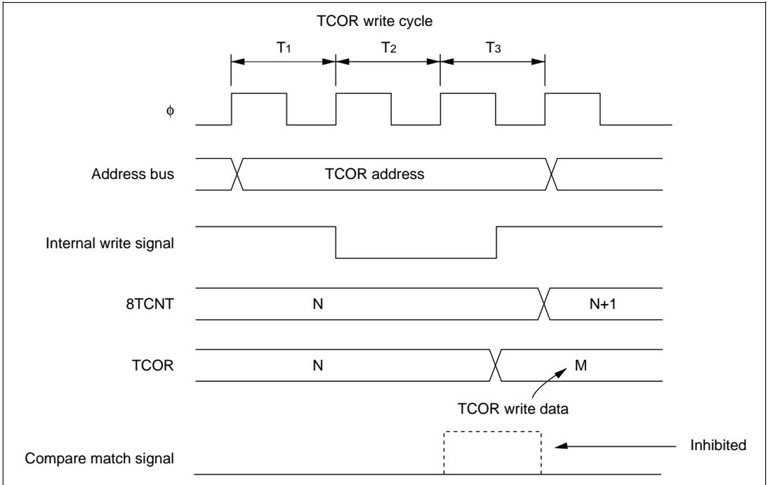
**Figure 10.20** Contention between TCOR Write and Compare Match
