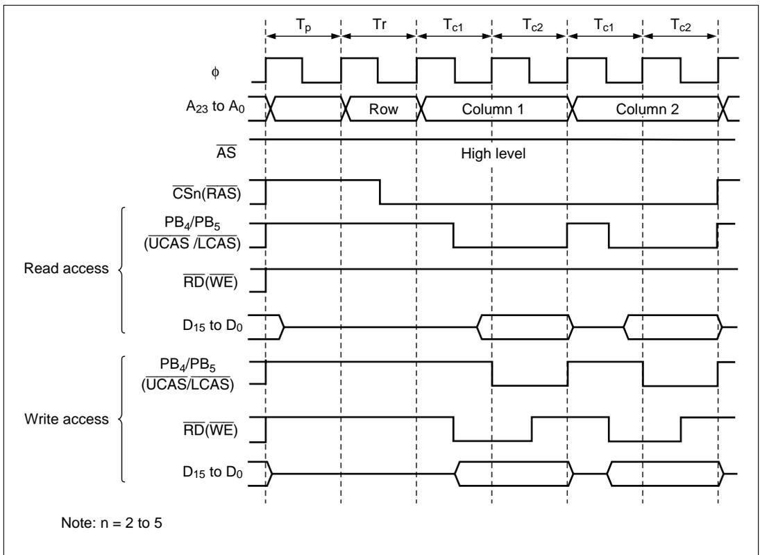
Figure 6.22 Operation Timing in Fast Page Mode
