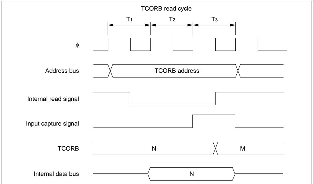
**Figure 10.21 Contention between TCOR Read and Input Capture**
