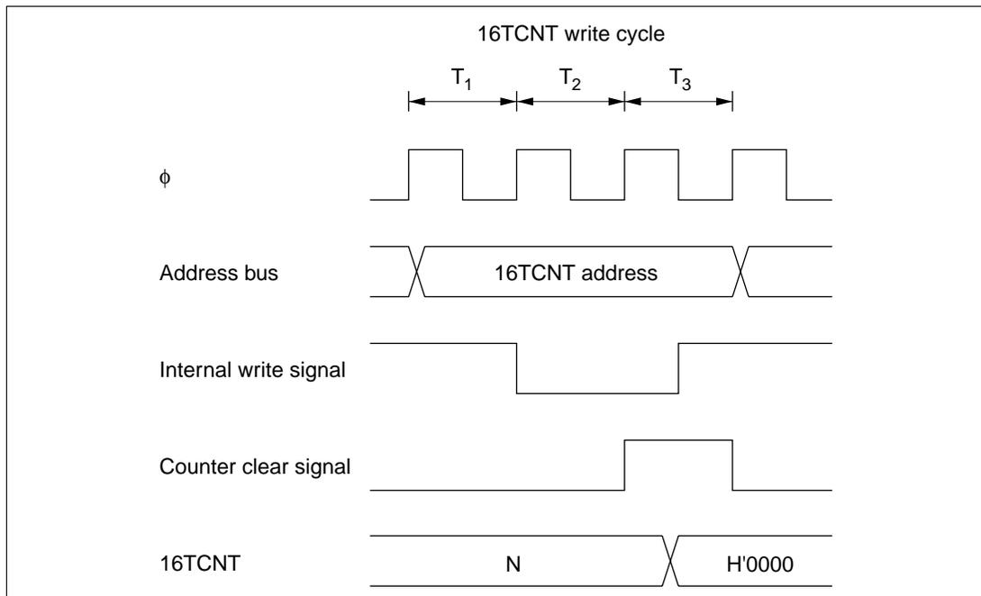
**Figure 9.37 Contention between 16TCNT Write and Clear**
