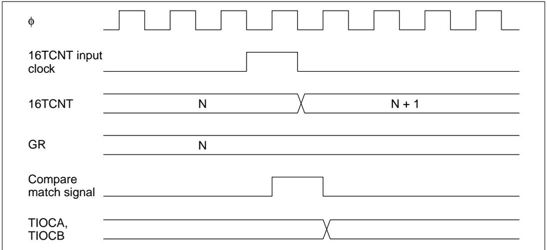
**Figure 9.20 Output Compare Output Timing**
