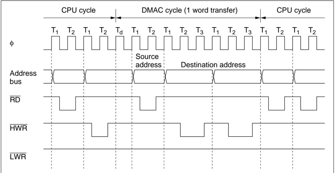
Figure 7.13 DMA Transfer Bus Timing (Example)
