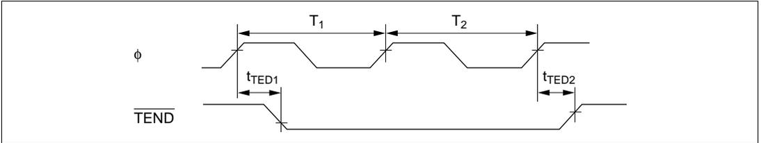
Figure 21.22 DMAC  $\overline{\text{TEND}}$  Output Timing for 2 State Access
