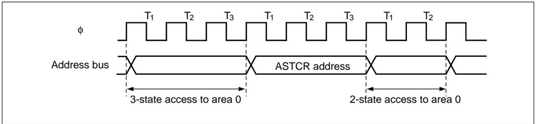
Figure 6.49 ASTCR Write Timing
