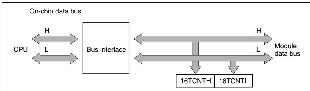
**Figure 9.4 16TCNT Access Operation [CPU → 16TCNT (Word)]**
