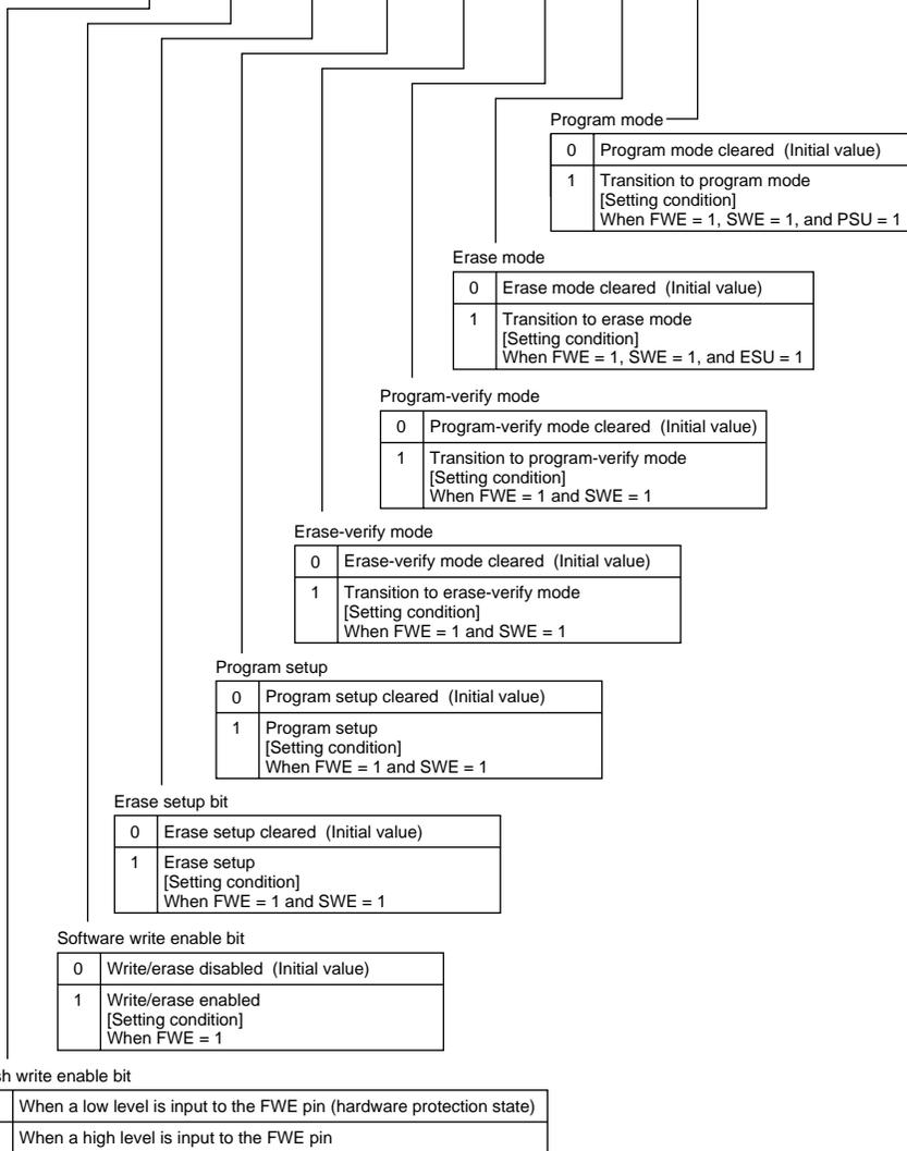
Note: This register is used only in the flash memory and flash memory R versions. Reading the corresponding address in a mask ROM version will always return 1s, and writes to this address are disabled. Fix the FWE pin low in mode 6.
