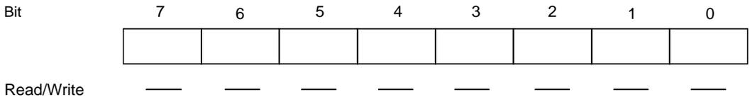
The SCI loads serial data input at the RxD pin into RSR in the order received, LSB (bit 0) first, thereby converting the data to parallel data. When one byte of data has been received, it is automatically transferred to RDR. The CPU cannot read or write RSR directly.
