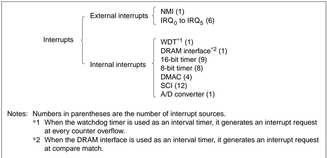
**Figure 4.5 Interrupt Sources and Number of Interrupts**
