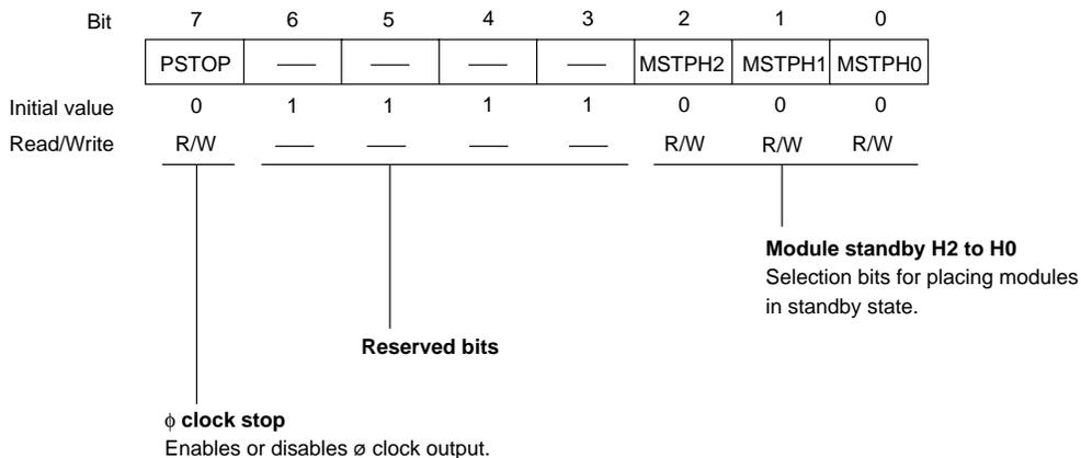
**MSTCRL—Module Standby Control Register L**
