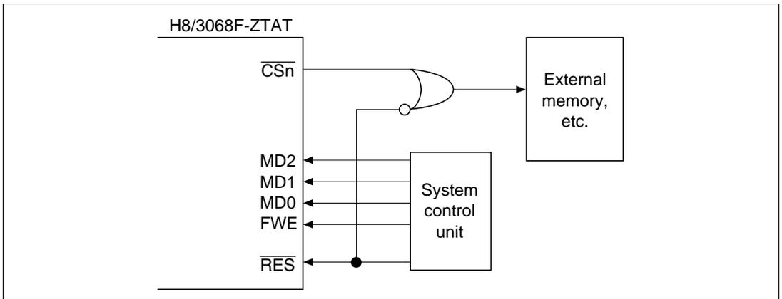
Notes: \*1 Mode pin and FWE pin input must satisfy the mode programming setup time ( $t_{\text{MDS}}$ ) with respect to the reset release timing.
