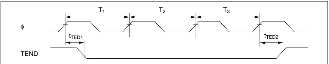
Figure 21.23 DMAC  $\overline{\text{TEND}}$  Output Timing for 3 State Access
