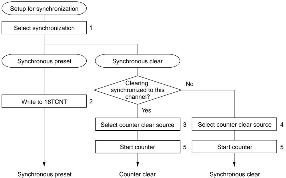
1. Set the SYNC bits to 1 in TSNC for the channels to be synchronized.
