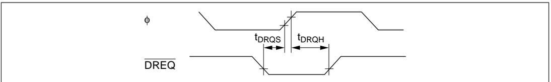
Figure 21.24 DMAC  $\overline{\text{DREQ}}$  Input Timing
