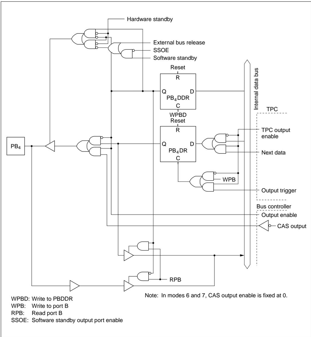
**Figure C.11 (e) Port B Block Diagram (Pin PB<sub>4</sub>)**
