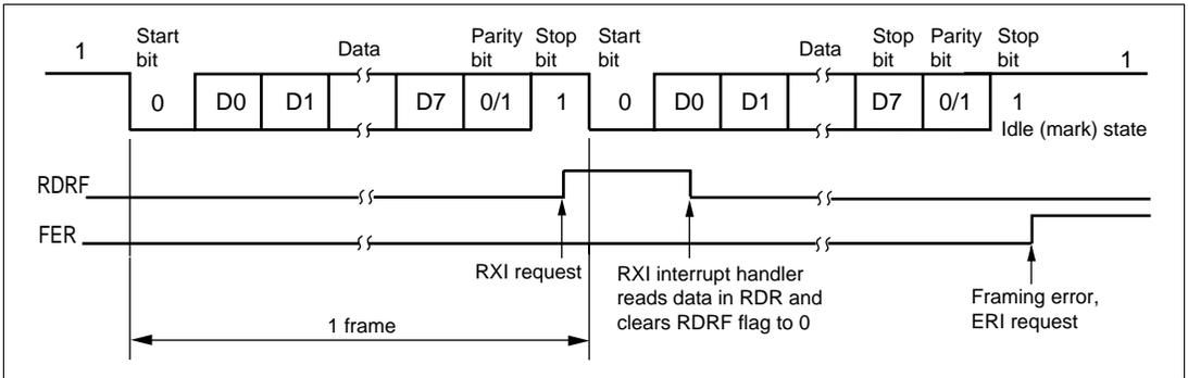
**Figure 13.8 Example of SCI Receive Operation
