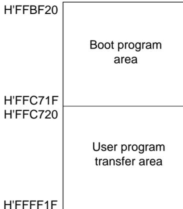
Note: The boot program area cannot be used until a transition is made to the execution state for the user program transferred to RAM. Note also that the boot program remains in this area in RAM even after control branches to the user program.
