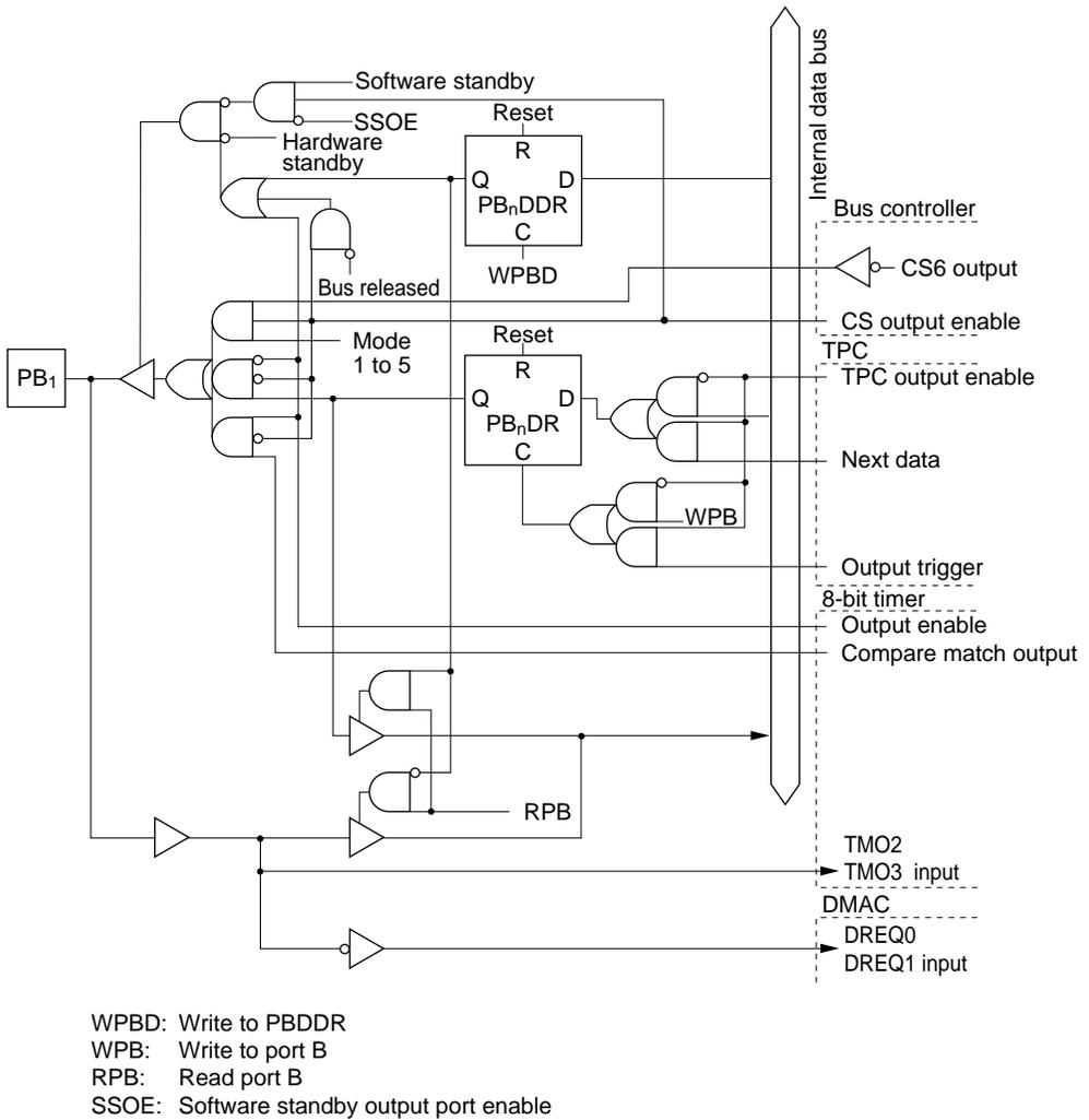
**Figure C.11 (b) Port B Block Diagram (Pin PB<sub>1</sub>)**
