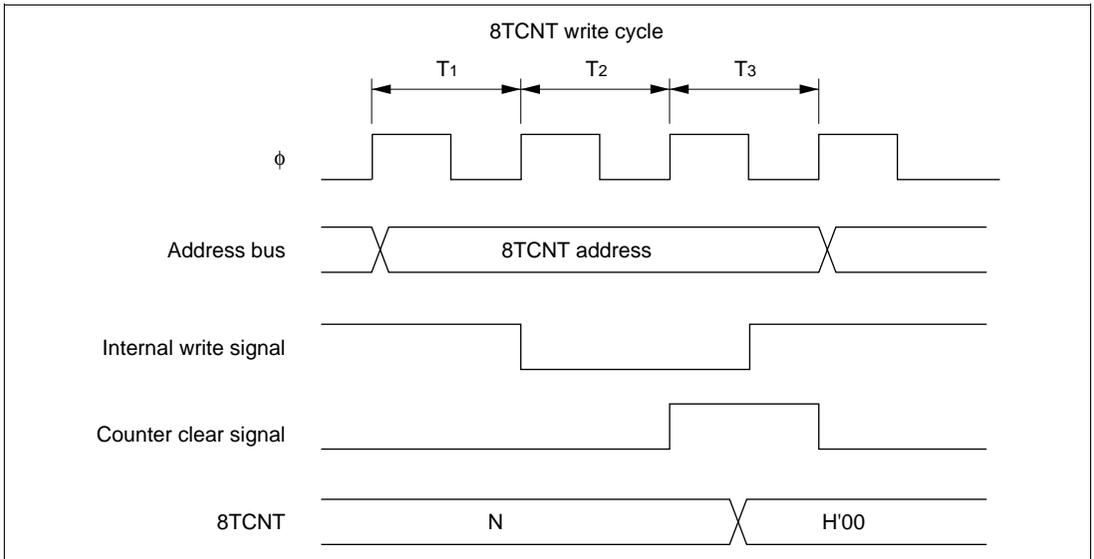
Figure 10.18 Contention between 8TCNT Write and Clear
