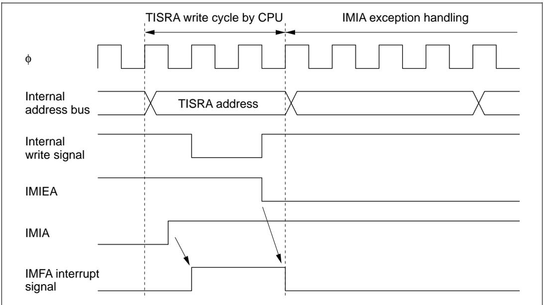
**Figure 5.8 Contention between Interrupt and Interrupt-Disabling Instruction**
