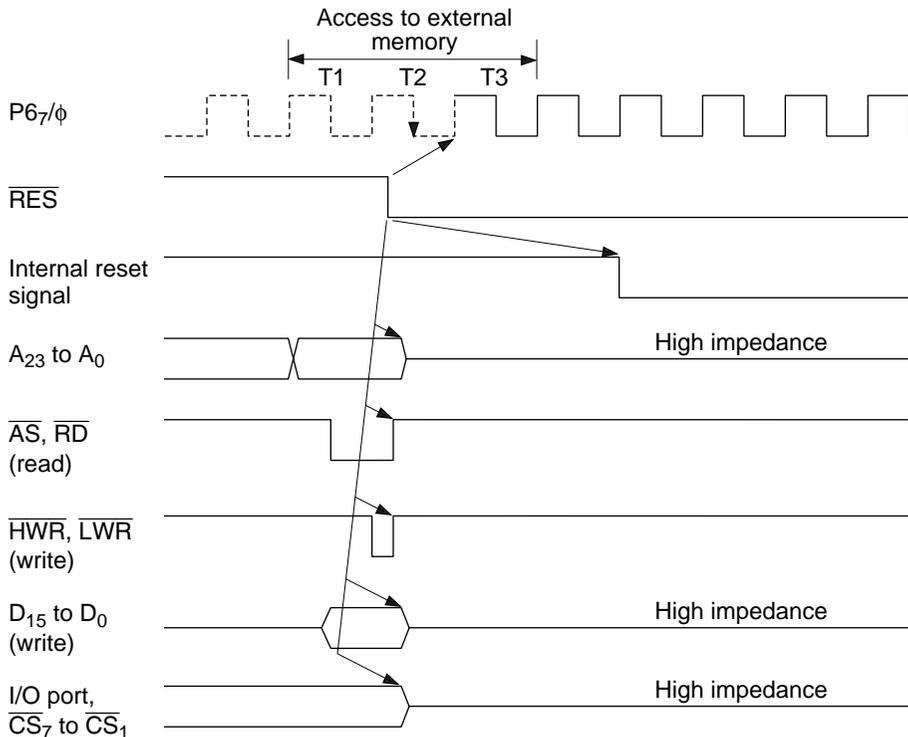
**Figure D.3 Reset during Memory Access (Mode 5)**
