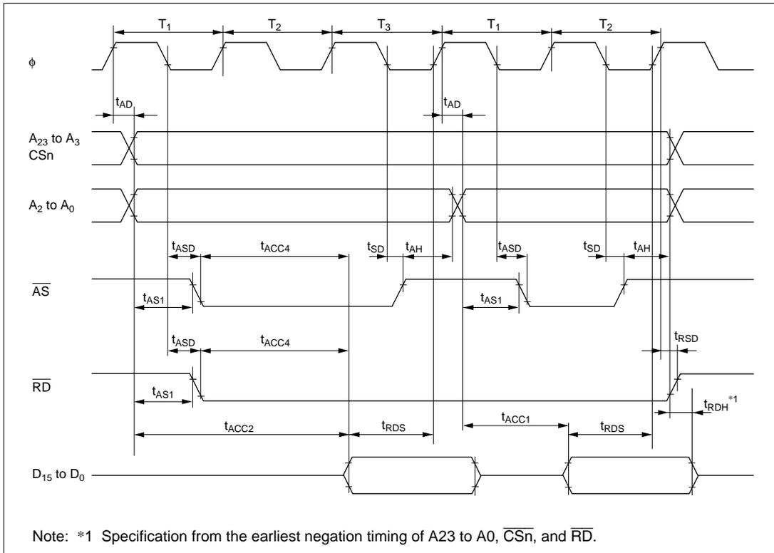
**Figure 21.11 Burst ROM Access Timing: Two-State Access**
