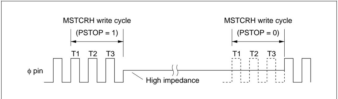
**Figure 20.3 Starting and Stopping of System Clock Output**
