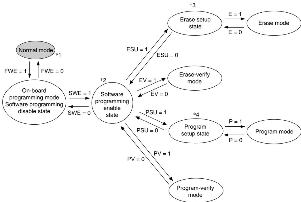
Notes: In order to perform a normal read of flash memory, SWE must be cleared to 0. Also note that verify-reads can be performed during the programming/erasing process.
