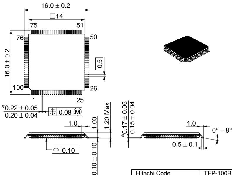
\*Dimension including the plating thickness
