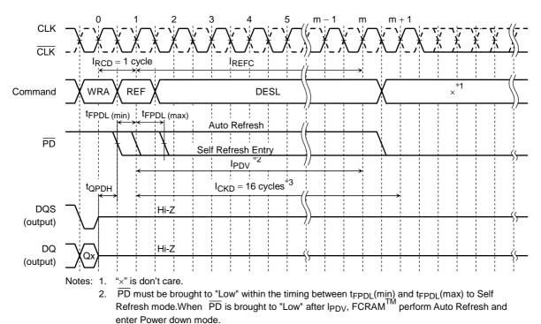
3. It is necessary that clock input is continued at least 16 clock cycles from REF command even though  $\overline{PD}$  is brought to "Low" for Self-Refresh Entry.
