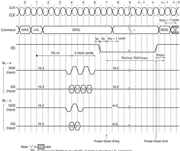
PD must be kept "High" level until WL+2 clock cycles from LAL command.
