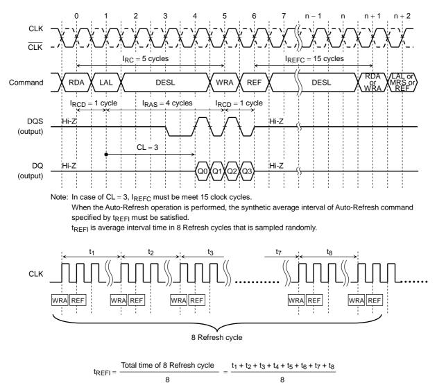
$t_{\mathsf{REFI}}$  is specified to avoid partly concentrated current of Refresh operation that is activated larger area than Read / Write operation.
