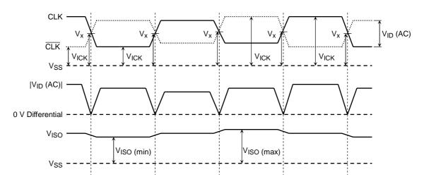
(11) In the case of external termination, VTT (termination voltage) should be gone in the range of VREF (DC)  $\pm$  0.04 V.
