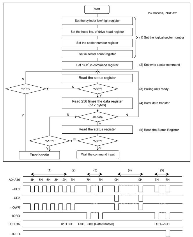
2. Sector write: write sector procedure after the card configured I/O interface is shown as follows.
