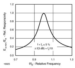
Fig. 5 - Frequency Dependence of Responsivity
