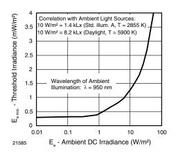
Fig. 6 - Sensitivity in Bright Ambient
