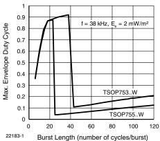
Fig. 9 - Max. Envelope Duty Cycle vs. Burst Length
