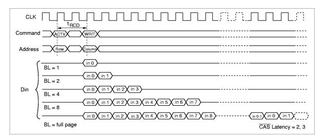
**2. Single write:** A single write operation is enabled by setting OPCODE (A9, A8) to (1, 0). In a single write operation, data is only written to the column address (AY0 to AY7; HM5264165D, AY0 to AY8; HM5264805D, AY0 to AY9; HM5264405D) and the bank select address (A12/A13) specified by the write command set cycle without regard to the burst length setting. (The latency of data input is 0 clock).
