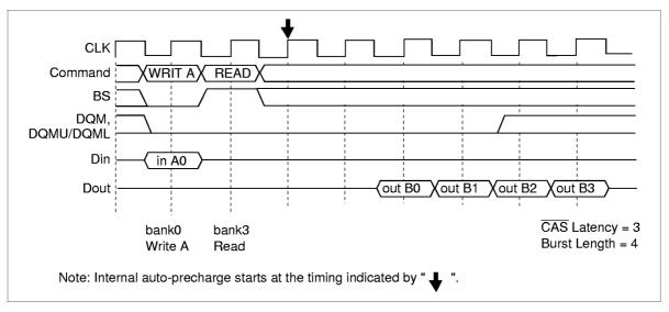
**Same bank:** The consecutive read command from write with auto precharge (the same bank) is illegal. . It is necessary to separate the two commands with a bank active command.
