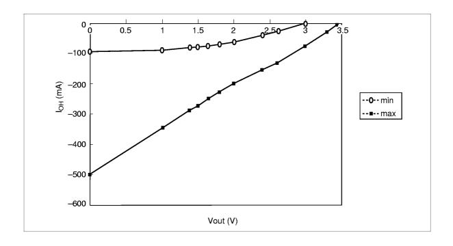
**DC Characteristics** (Ta = 0 to 70°C,  $V_{CC}$ ,  $V_{CC}Q = 3.3 \text{ V} \pm 0.3 \text{ V}$ ,  $V_{SS}$ ,  $V_{SS}Q = 0 \text{ V}$ ) (HM5264165D)
