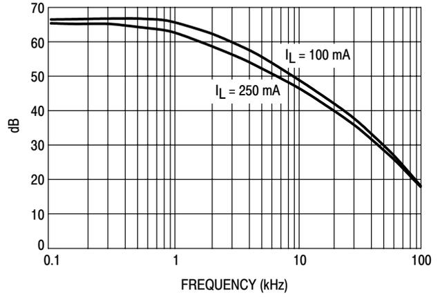
Figure 13. Ripple Rejection
