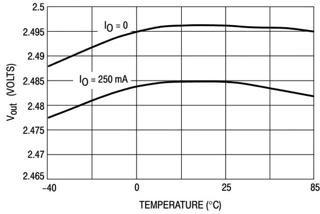
Figure 11. Output Voltage versus Ambient Temperature ( $V_{in} = 12$  V)
