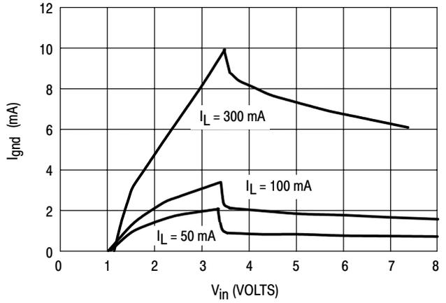
Figure 8. Ground Pin Current versus Input Voltage
