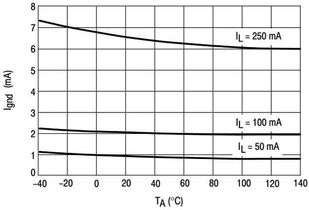
Figure 9. Ground Pin Current versus Ambient Temperature
