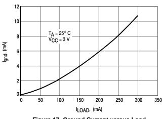
Figure 17. Ground Current versus Load Current
