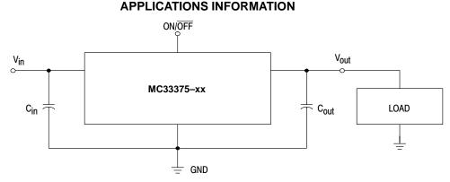
Figure 22. Typical Application Circuit
