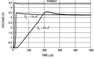
Figure 14. Enable Transient
