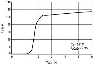
Figure 18. Quiescent Current versus Input Voltage
