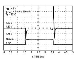
Figure 21. Load Transient Response
