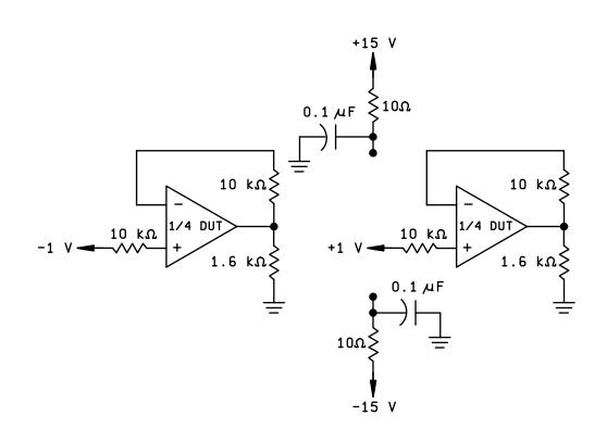
FIGURE 2. Radiation exposure circuit.
