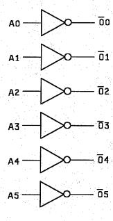
FIGURE 3. Logic diagram.
