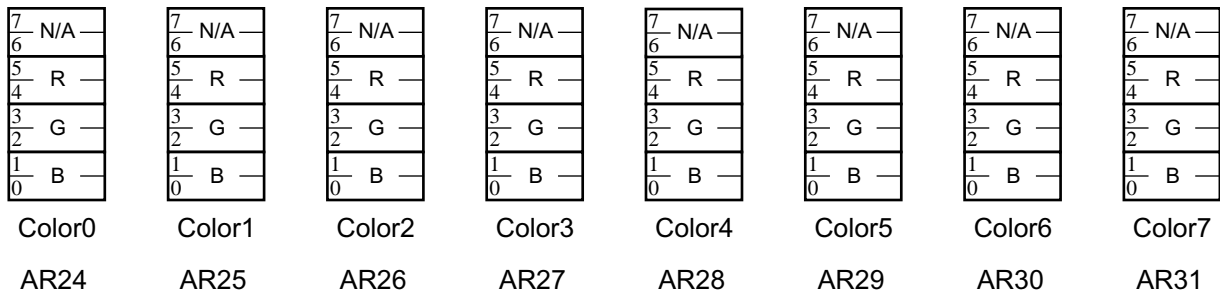
Figure 24 Programmable Palette Control at AR Register
