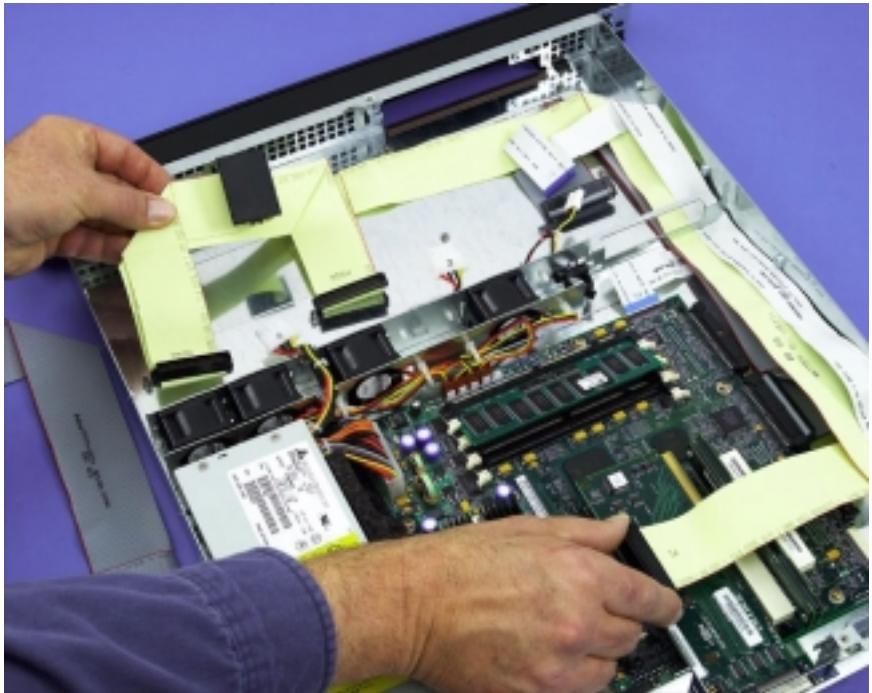
Figure 13 SCSI Cable Routing
