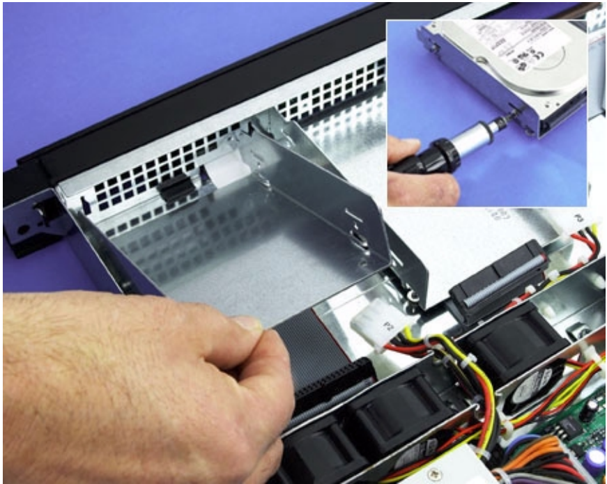
Figure 11 Removing the Hard Drive Bays
