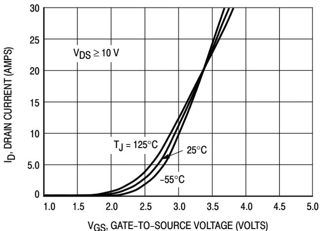
Figure 2. Transfer Characteristics
