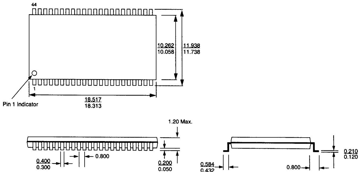
Measurements are in Millimeters unless otherwise specified.  $(\frac{\text{MAX}}{\text{MIN}})$
