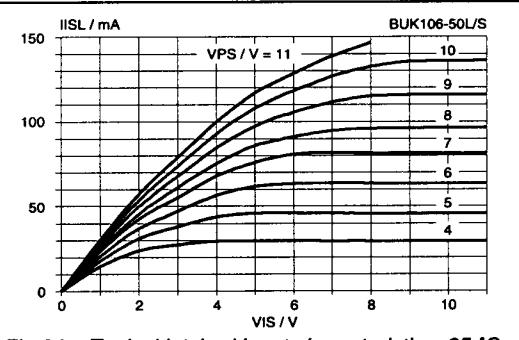
Fig.24. Typical latched input characteristics,  $25^\circ\text{C}$ .
