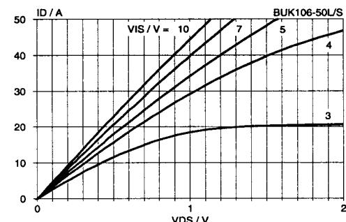
Fig.9. Typical on-state characteristics,  $T_j = 25^\circ\text{C}$ .
