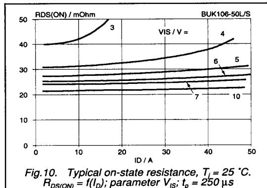
Fig.10. Typical on-state resistance,  $T_j = 25^\circ\text{C}$ .
