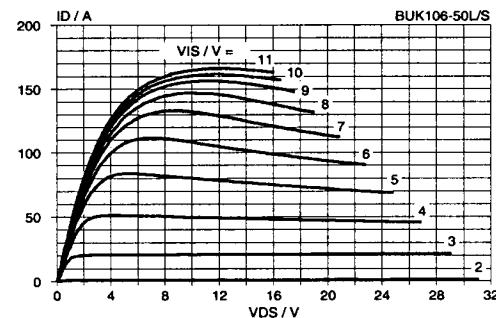
Fig.8. Typical output characteristics,  $T_j = 25^\circ\text{C}$ .
