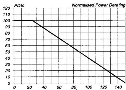
Fig.4. Normalised limiting power dissipation.
