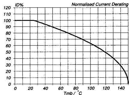
Fig.5. Normalised continuous drain current.
