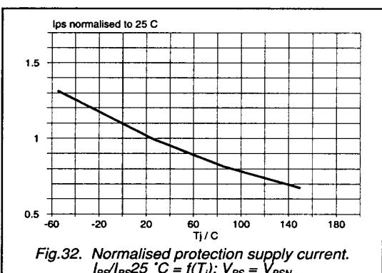
Fig.32. Normalised protection supply current.
