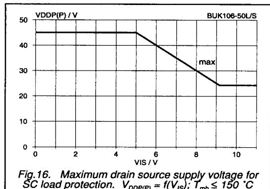
Fig.16. Maximum drain source supply voltage for SC load protection.  $V_{DDP(P)} = f(V_{IS})$ ;  $T_{mb} \leq 150^\circ\text{C}$
