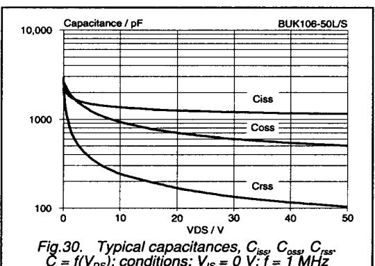
Fig.30. Typical capacitances,  $C_{iss}$ ,  $C_{oss}$ ,  $C_{rss}$ .
