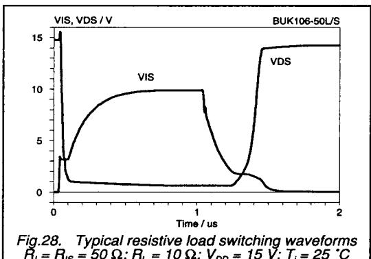
Fig.28. Typical resistive load switching waveforms.
