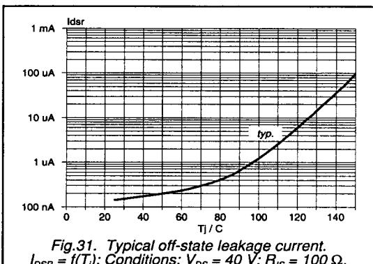
Fig.31. Typical off-state leakage current.
