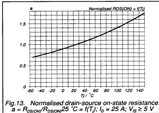
Fig.13. Normalised drain-source on-state resistance.
