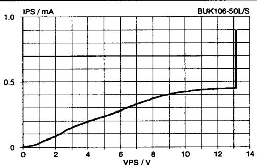
Fig.23. Typical DC protection supply characteristics.
