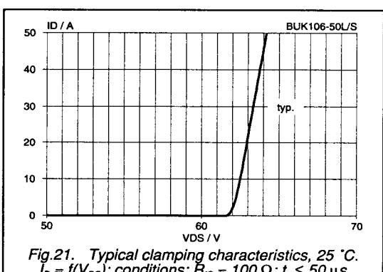
Fig.21. Typical clamping characteristics,  $25^\circ\text{C}$ .  $I_D = f(V_{DS})$ ; conditions:  $R_{IS} = 100\Omega$ ;  $t_p \leq 50\mu\text{s}$
