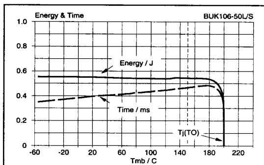
Fig.19. Typical overload protection characteristics. Conditions:  $V_{DD} = 13\text{ V}$ ;  $V_{PS} = V_{PSN}$ ;  $V_{IS} = 8\text{ V}$ ; SC load
