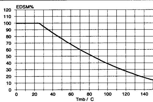
Fig.26. Normalised limiting clamping energy.
