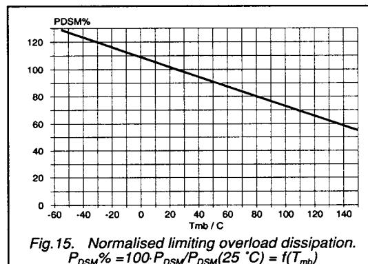
Fig.15. Normalised limiting overload dissipation.
