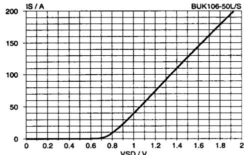
Fig.25. Typical reverse diode current,  $T_J = 25^\circ\text{C}$ .
