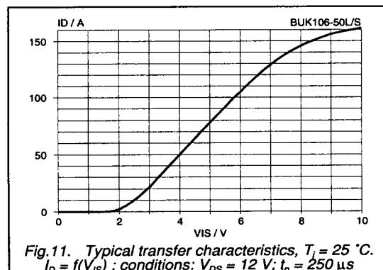
Fig.11. Typical transfer characteristics,  $T_j = 25^\circ\text{C}$ .
