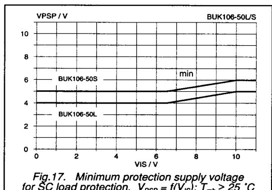
Fig.17. Minimum protection supply voltage for SC load protection.  $V_{PS} = f(V_{IS})$ ;  $T_{mb} \geq 25^\circ\text{C}$
