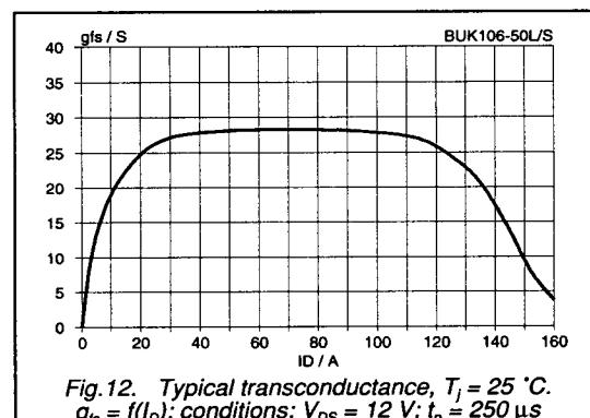
Fig.12. Typical transconductance,  $T_j = 25^\circ\text{C}$ .
