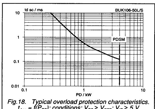
Fig.18. Typical overload protection characteristics.  $t_{d sc} = f(P_{DS})$ ; conditions:  $V_{PS} \geq V_{PSP}$ ;  $V_{IS} \geq 5\text{ V}$
