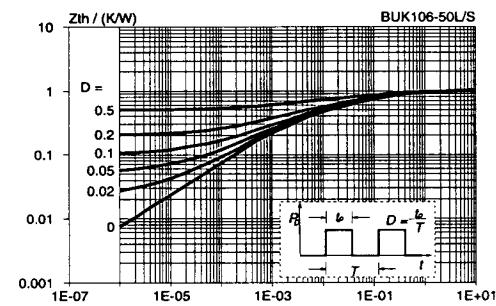
Fig.7. Transient thermal impedance.
