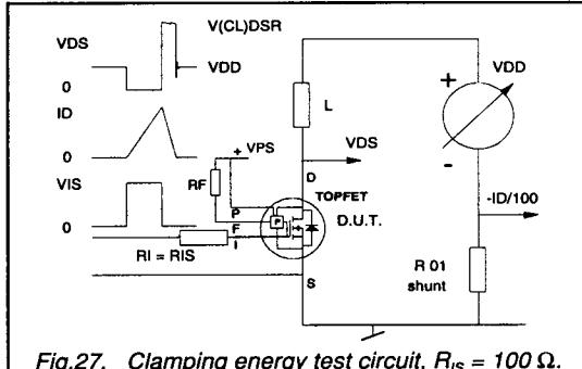
Fig.27. Clamping energy test circuit,  $R_{IS} = 100 \Omega$ .
