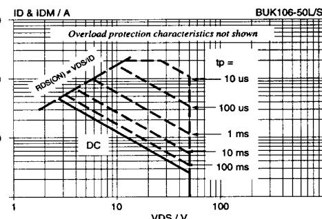
Fig.6. Safe operating area,  $T_{mb} = 25^\circ\text{C}$
