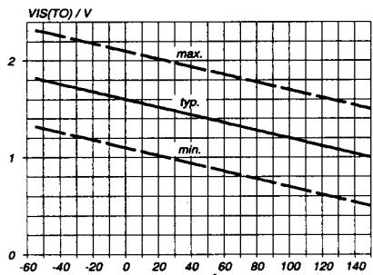
Fig.22. Input threshold voltage.
