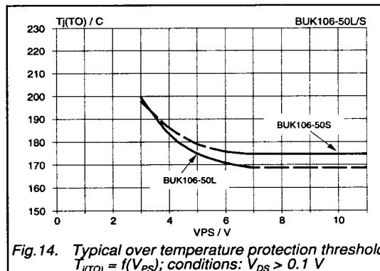
Fig.14. Typical over temperature protection threshold
