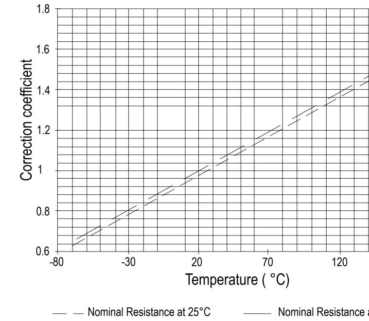
Example: Coil resistance at 25°C: 935 ohms. What is it at 125°C?
