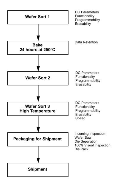
Figure 1. AMD KGD Product Test Flow
