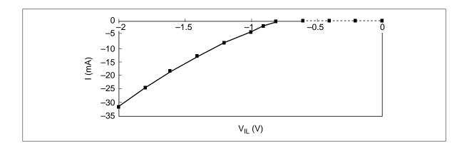
$\label{eq:minimum} \textbf{Minimum} \ \textbf{V}_{\textbf{IH}} \ \textbf{Clamp} \ \textbf{Current} \ (\text{referred to} \ V_{\text{IH}})$
