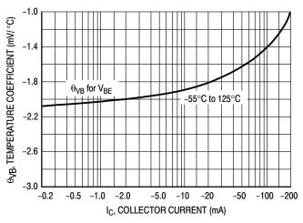
Figure 4. Base-Emitter Temperature Coefficient
