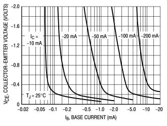
**Figure 3. Collector Saturation Region**
