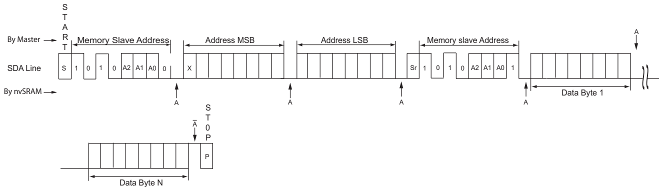
Figure 21. Random Address Single-Byte Read (Hs-mode)
